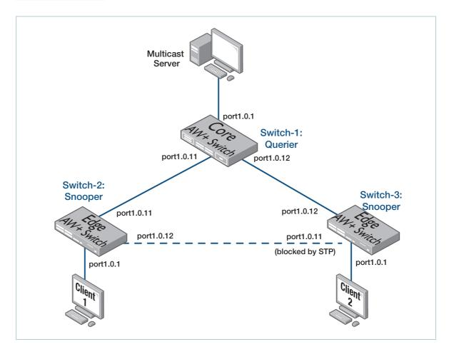
Step 1. Configure Switch-1, the IGMP/MLD Querier
