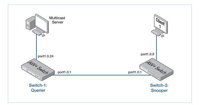
The example considers what happens when a port comes up. When the port was down, the client stopped receiving multicasts because there was no backup route available. The example shows how the network recovers. The multicast group is 224.12.13.14.
