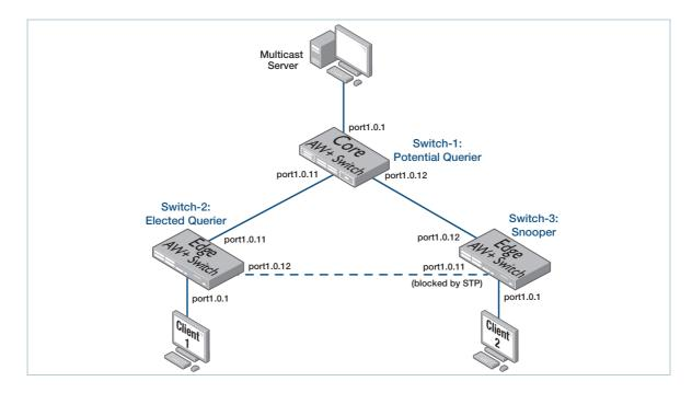
Both Switch-1 and Switch-2 are configured with IGMP/MLD, making both of them potential Queriers. Switch-3, by default configuration, is an IGMP/MLD Snooper.
