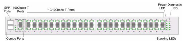
The AT-8000S/48 device front panel is configured as follows:
