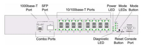
The AT-8000S/16 front panel is configured as follows:
