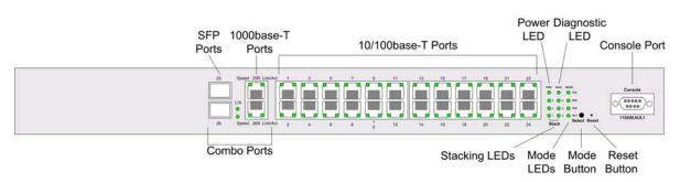
The AT-8000S/24 front panel is configured as follows:
