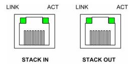
The RJ-45 ports have two LEDs, one is for link and one is for activity. The Stacking LEDs indications are described in the following table:
