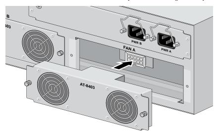
3. Fasten the two Phillips-head screws on the top of the fan as shown below.
