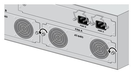
2. Insert the new fan into the Fan A or Fan B slot at the rear of the chassis, as shown below. Check that the AT-8403 part number is right-side up.
