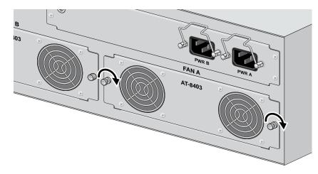
WARNING: To avoid electric shock, do not place fingers or hands inside fan slot.
