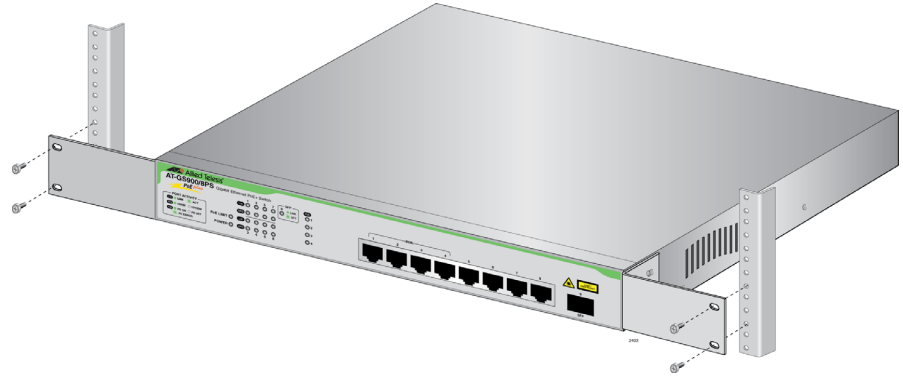
Figure 7. Mounting the Switch in an Equipment Rack
