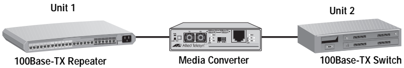
Figure 3 Example of a Duplex Mode Mismatch
