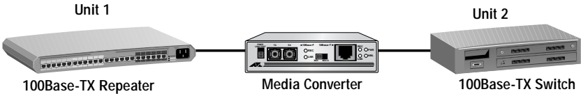
Figure 1 Example of a Duplex Mode Mismatch
