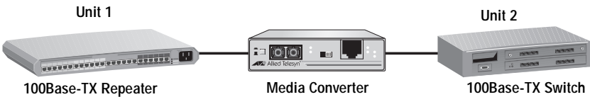
Figure 3 Example of a Duplex Mode Mismatch
