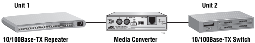
Figure 3. Example of a Duplex Mode Mismatch
