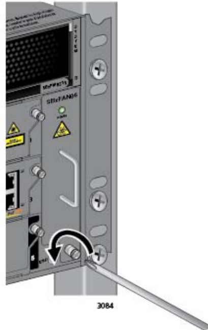
Figure 190. Loosening the Screw on the AT-SBx31CFC960 Card
