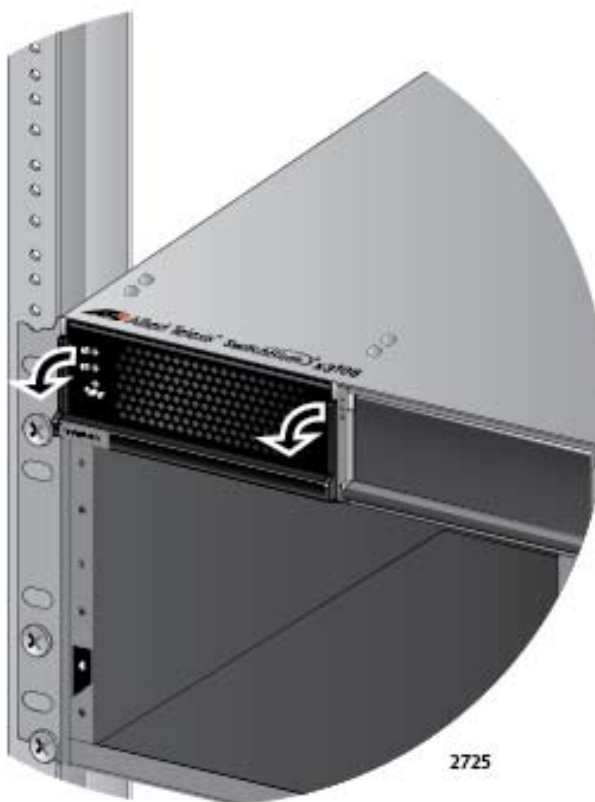
Figure 65. Locking the Handle on the AT-SBxPWRPOE1 AC Power Supply
