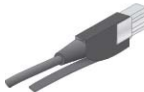
Figure 99. Connecting Cables to Ports on the AT-SBx31GT40 Line Card
