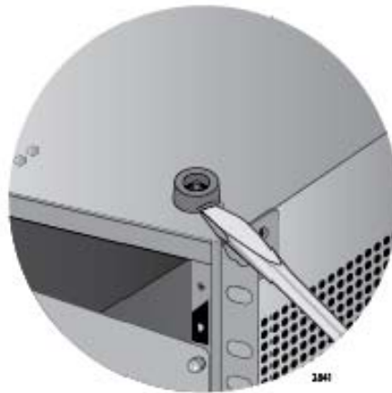
Figure 43. Removing the Rubber Feet
