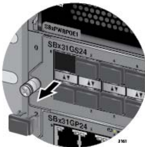
Figure 100. Removing the Dust Cover from an SFP Slot in the AT-SBx31GS24 Line Card
