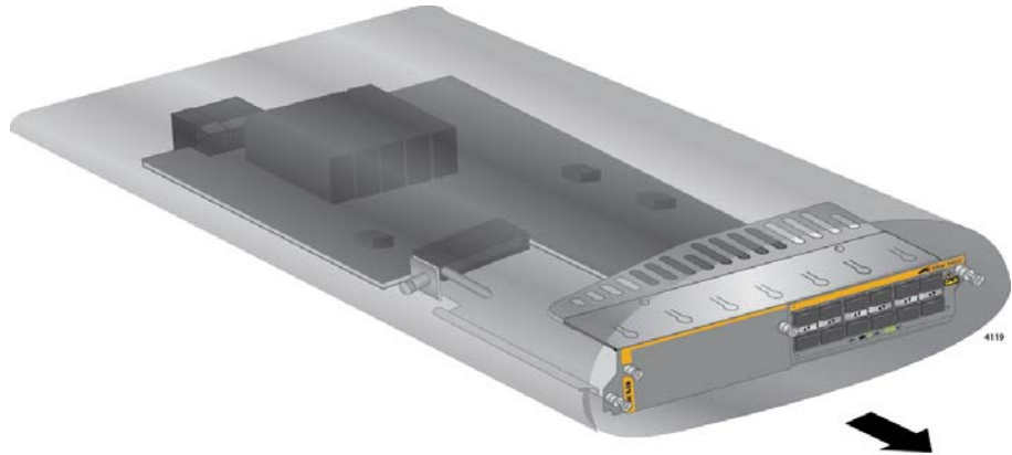
Figure 81. Removing the AT-SBx81XLEM Line Card from the Anti-static Bag
