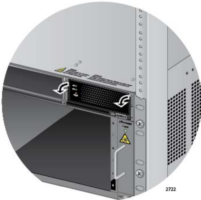
Figure 60. Lowering the Handle on the AT-SBxPWRSYS1 or AT-SBxPWRSYS2 AC Power Supply
