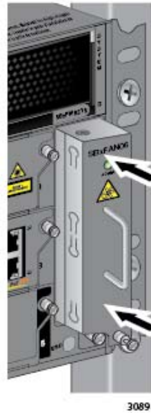
Figure 195. Securing the AT-SBxFAN06 Fan Module on the Backplane Connector
