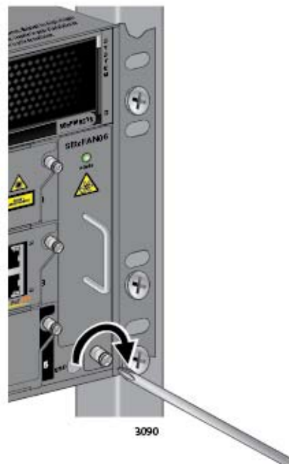
Figure 196. Tightening the Screw on the AT-SBxFAN06 Fan Module
