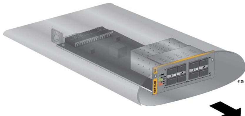
Figure 85. Removing the Expansion Module from the Anti-static Bag
