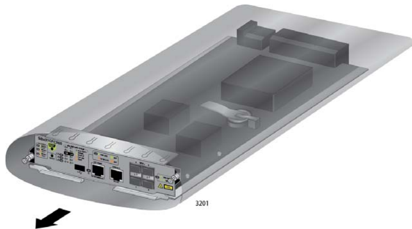
Figure 75. Removing the AT-SBx31CFC960 Controller Fabric Card from the Anti-static Bag
