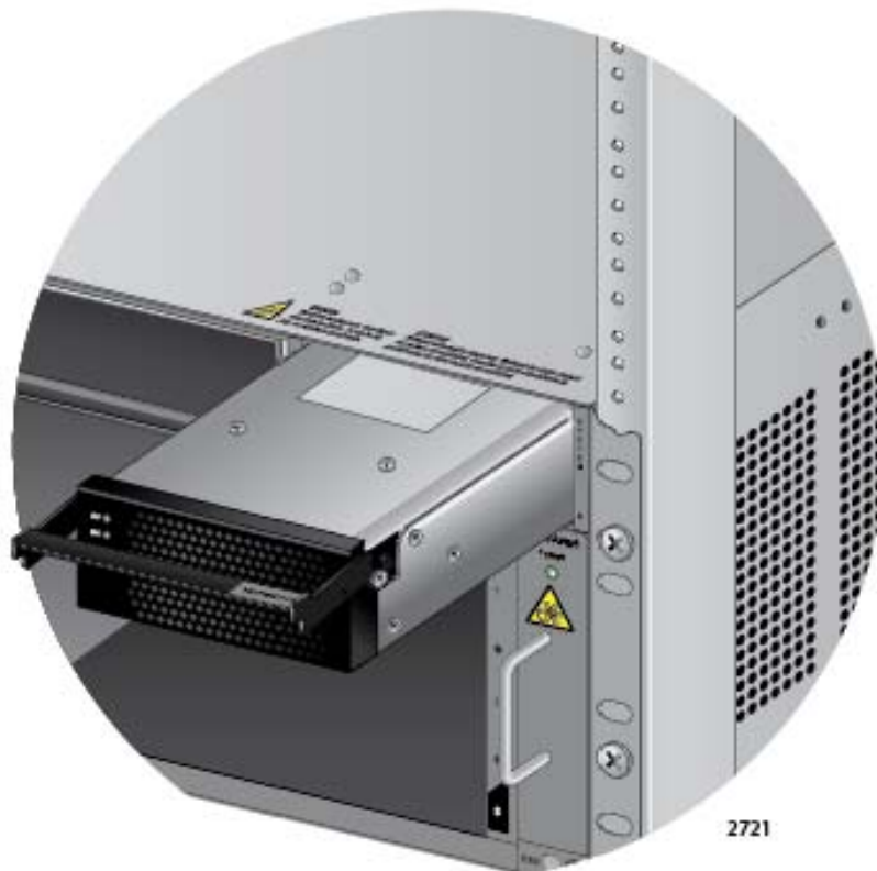
Figure 59. Inserting the AT-SBxPWRSYS1 AC or AT-SBxPWRSYS2 Power Supply
