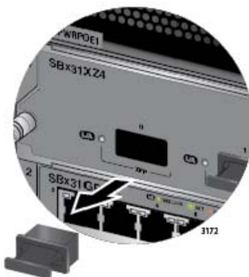
Figure 107. Removing the Dust Cover From an XFP Slot on the AT-SBx31XZ4 Line Card
