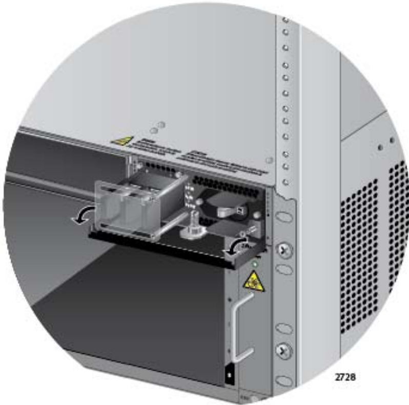
Figure 71. Locking the Handle on the AT-SBxPWRSYS1 DC System Power Supply
