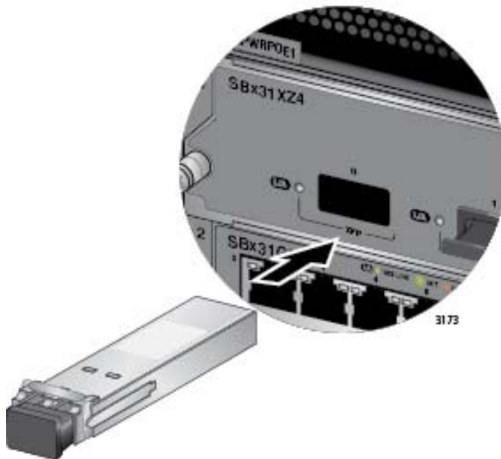
Figure 109. Installing an XFP Transceiver in the AT-SBx31XZ4 Line Card
