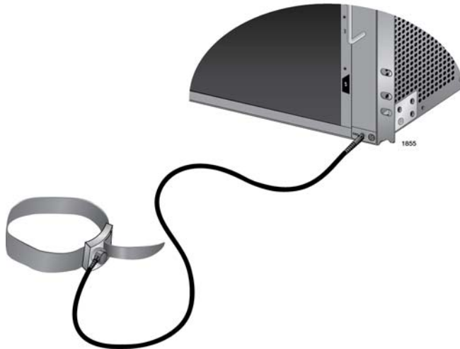
Figure 54. ESD Socket and Wrist Strap
