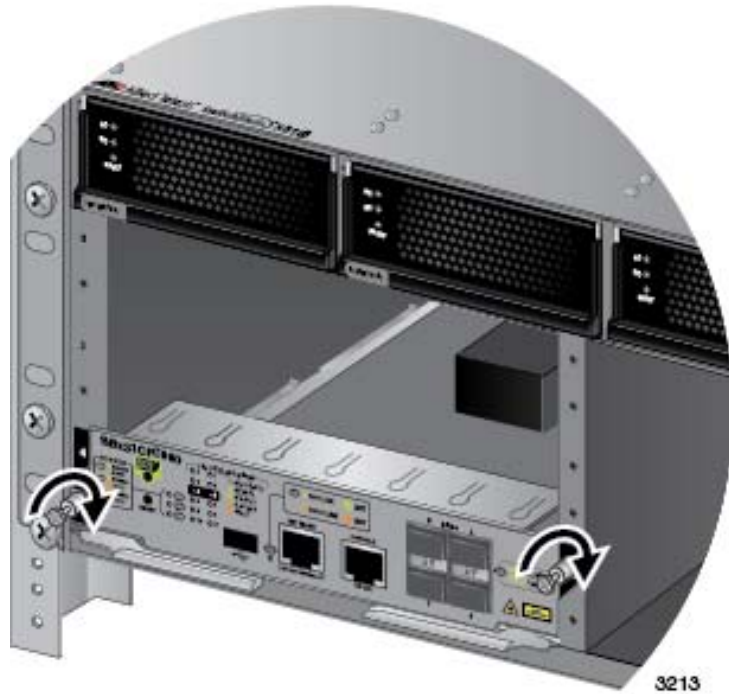
Figure 80. Tightening the Thumb Screws on the AT-SBx31CFC960 Card
