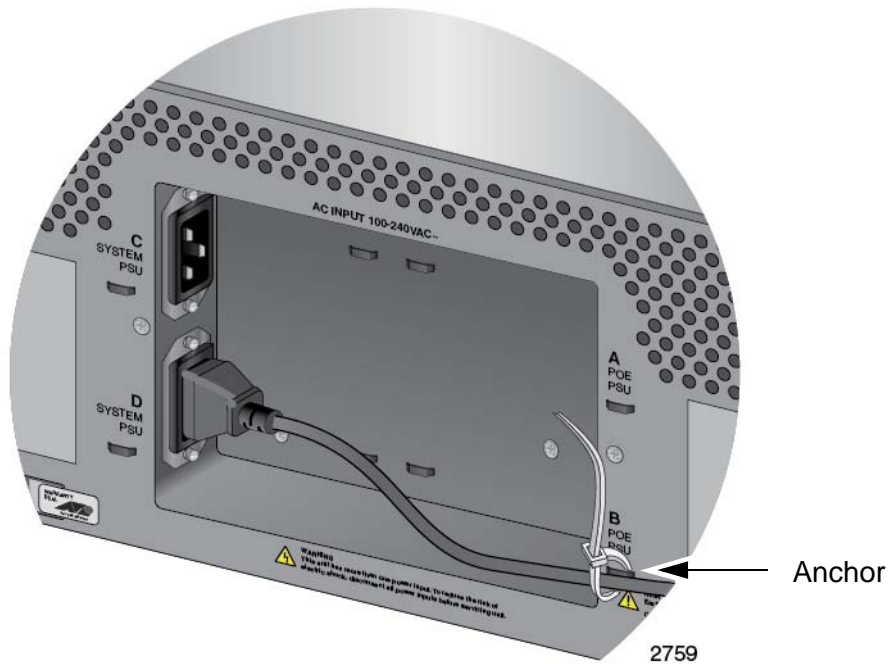
Figure 121. Securing the Power Cord for the AT-SBxPWRSYS1 or AT-SBxPWRSYS2 AC System Power Supply to an Anchor
