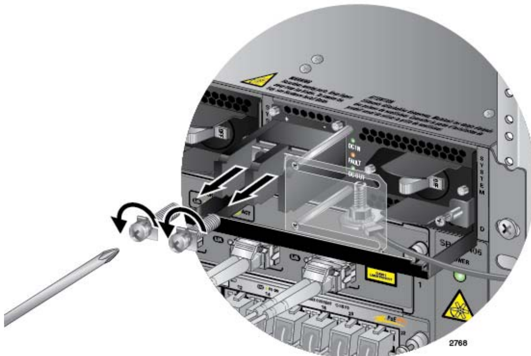
Figure 139. Removing the Terminal Screws
