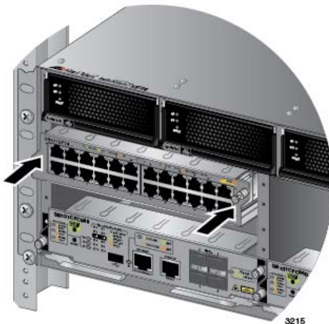
Figure 94. Seating an Ethernet Line Card on the Backplane Connector
