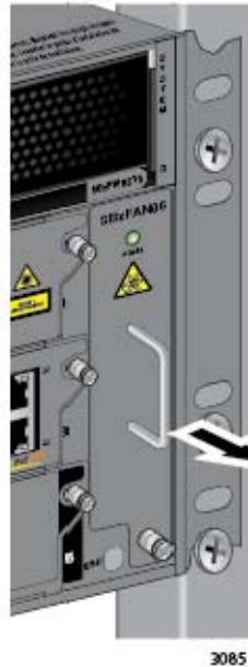
Figure 191. Loosening the AT-SBx31CFC960 Fan Module from the Backplane Connector
