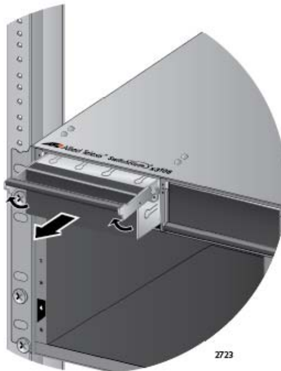
Figure 61. Removing the Blank Slot Cover from Power Supply Slot A
