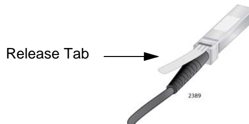
Figure 99. Release Tab on the AT-SBx31XS6 Line Card
