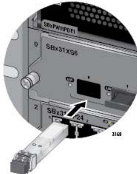
Figure 96. Installing an SFP+ Transceiver in the AT-SBx31XS6 Line Card
