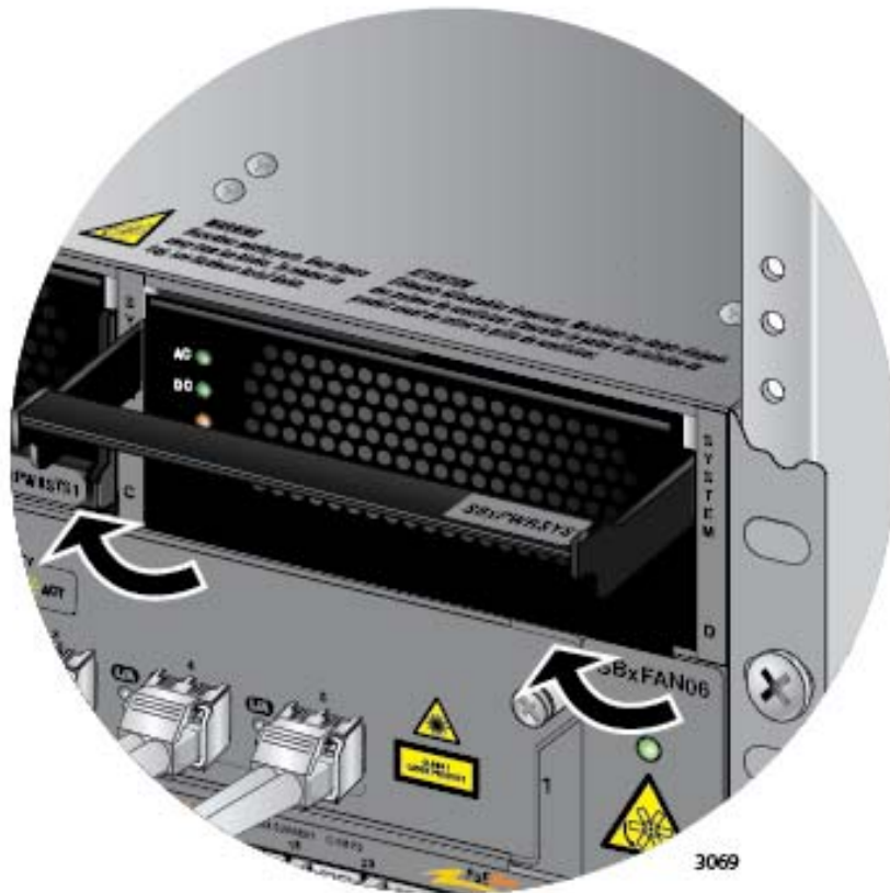
Figure 148. Lifting the Locking Handle on the Power Supply
