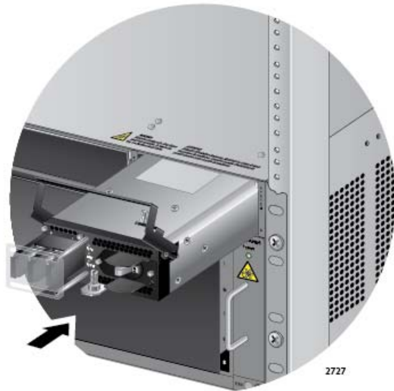
Figure 65. Inserting the AT-SBxPWRSYS1 DC System Power Supply
