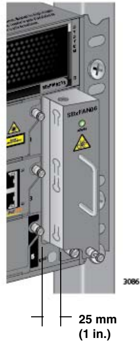
Figure 165. Withdrawing the AT-SBxFAN06 Fan Module 25 mm (1 in.) from the Chassis
