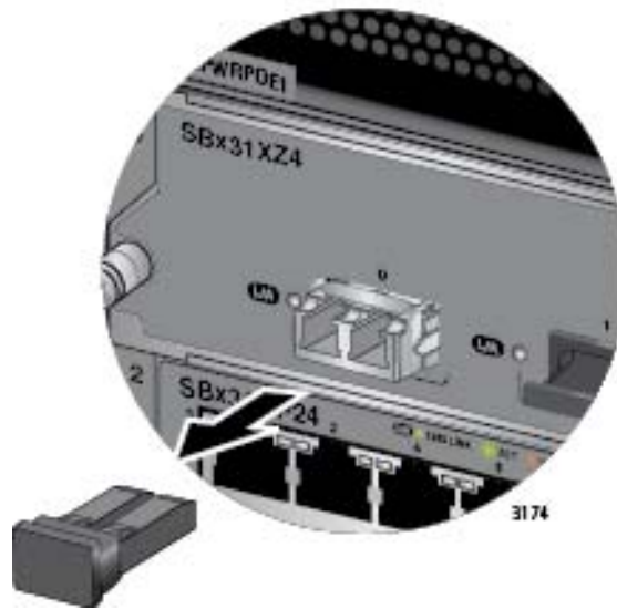
Figure 104. Removing the Protective Cover from an XFP Transceiver in the AT-SBx31XZ4 Line Card
