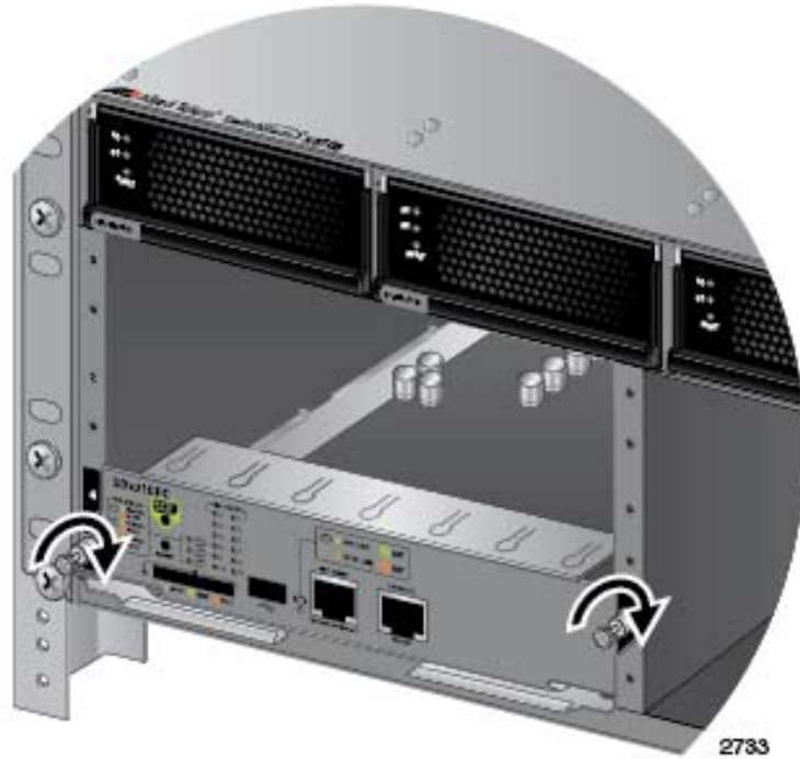
Figure 75. Tightening the Thumb Screws on the AT-SBx31CFC Card
