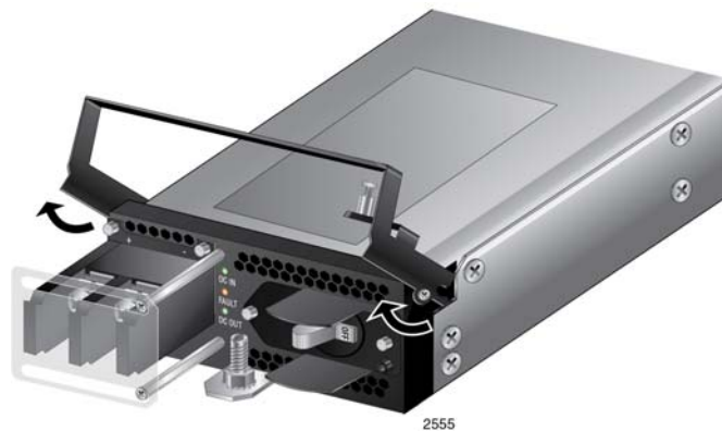
Figure 64. Raising the Handle on the AT-SBxPWRPOE1 DC System Power Supply
