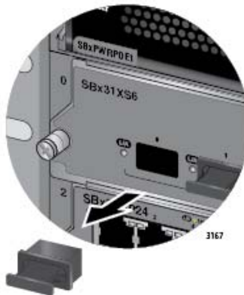
Figure 94. Removing a Dust Cover From an SFP+ Slot in the AT-SBx31XS6 Line Card
