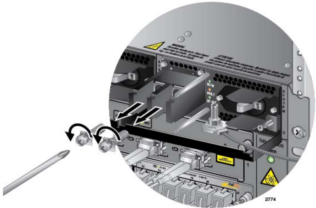
Figure 134. Removing the Terminal Screws
