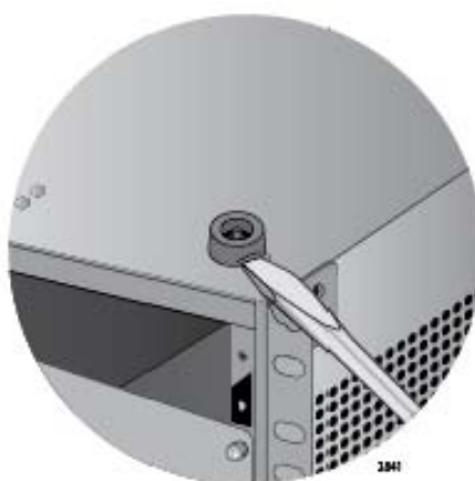
Figure 38. Removing the Rubber Feet
