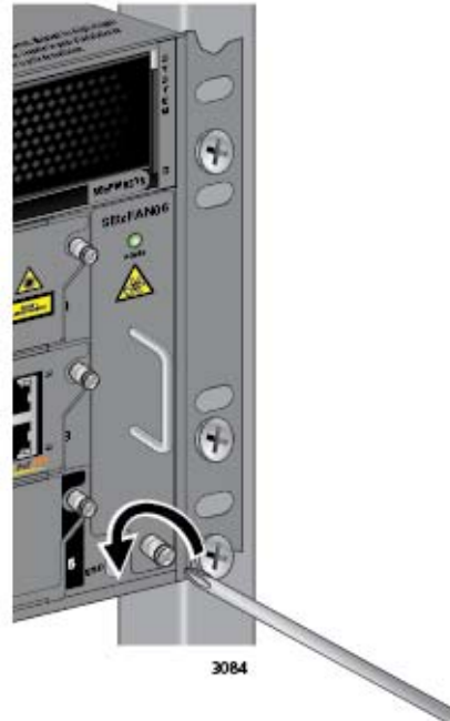
Figure 163. Loosening the Screw on the AT-SBx31CFC Fan Module
