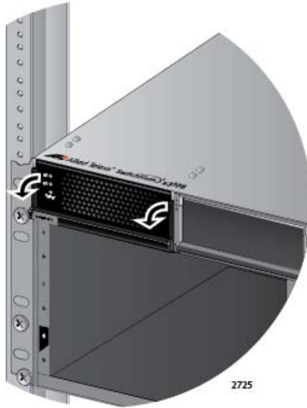
Figure 60. Locking the Handle on the AT-SBxPWRPOE1 AC Power Supply
