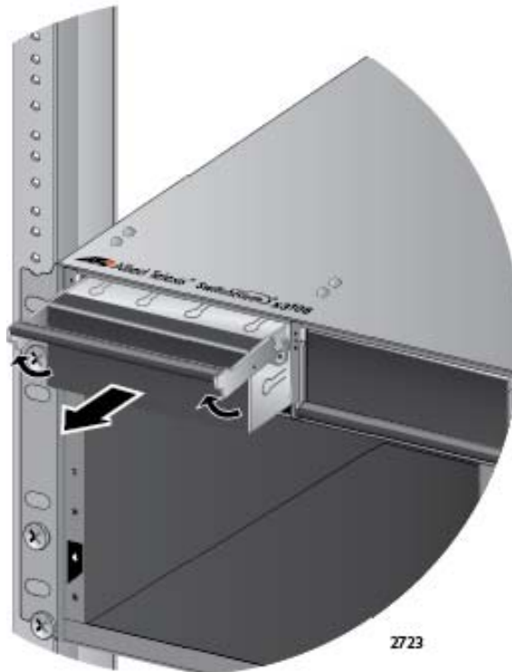
Figure 56. Removing the Blank Slot Cover from Power Supply Slot A
