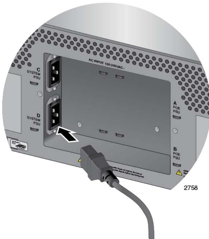
Figure 107. Connecting the AC Power Cord for the AT-SBxPWRSYS1 or AT-SBxPWRSYS2 AC System Power Supply
