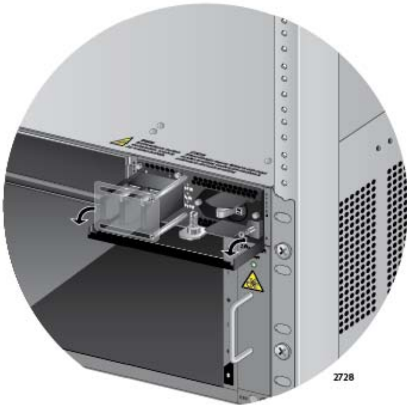
Figure 66. Locking the Handle on the AT-SBxPWRSYS1 DC System Power Supply
