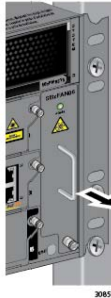
Figure 164. Loosening the AT-SBx31CFC Fan Module from the Backplane Connector
