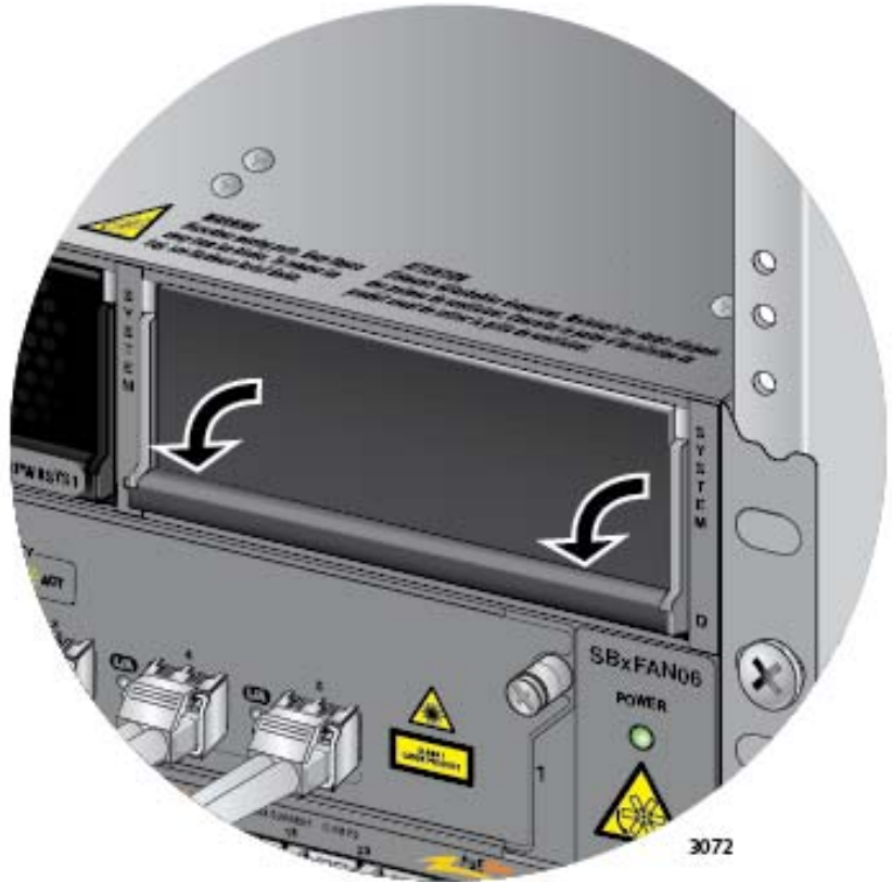
Figure 151. Lowering the Locking Handle on the Power Supply Slot Cover
