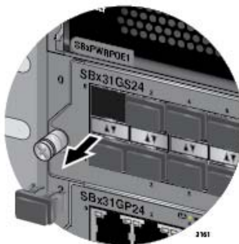
Figure 84. Removing the Dust Cover from an SFP Slot in the AT-SBx31GS24 Line Card
