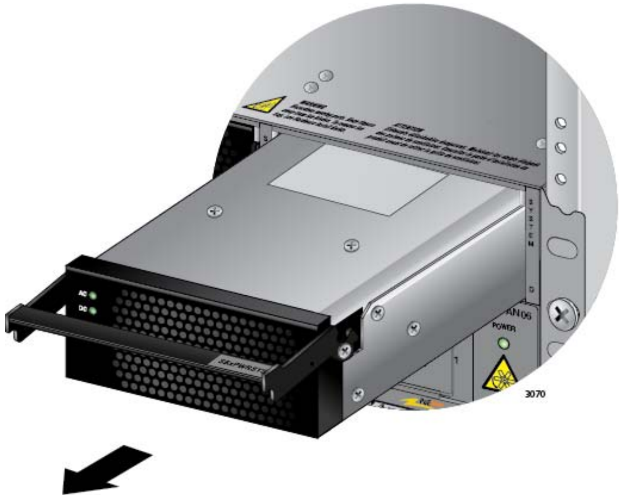
Figure 149. Removing the Power Supply from the Chassis
