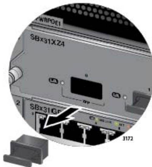
Figure 101. Removing the Dust Cover From an XFP Slot on the AT-SBx31XZ4 Line Card
