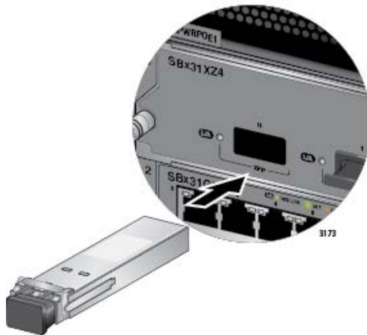
Figure 103. Installing an XFP Transceiver in the AT-SBx31XZ4 Line Card
