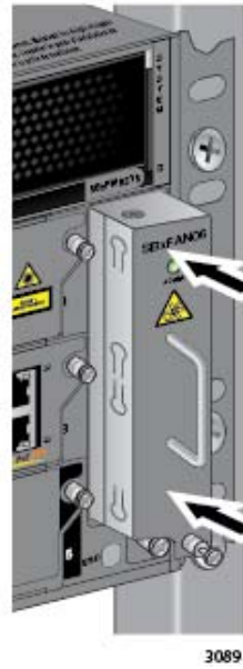
Figure 168. Securing the AT-SBx31CFC Fan Module on the Backplane Connector
