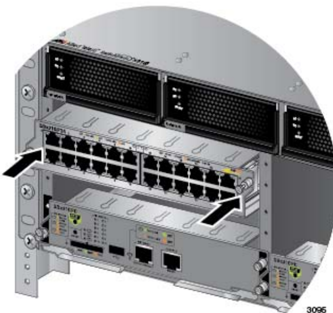
Figure 78. Seating an Ethernet Line Card on the Backplane Connector
