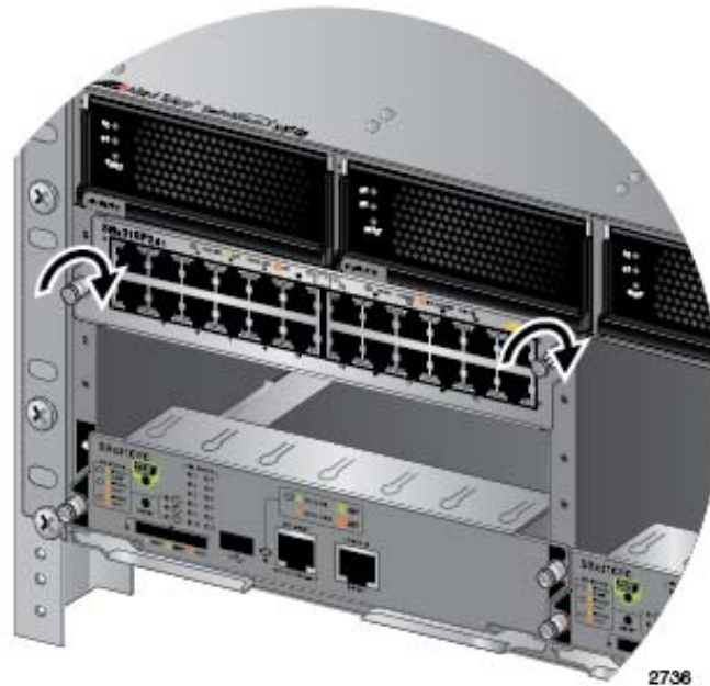
Figure 79. Tightening the Thumb Screws on an Ethernet Line Card
