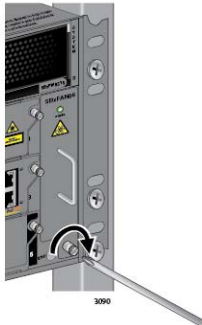
Figure 169. Tightening the Screw on the AT-SBx31CFC Fan Module
