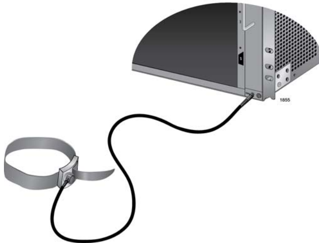
Figure 49. ESD Socket and Wrist Strap
