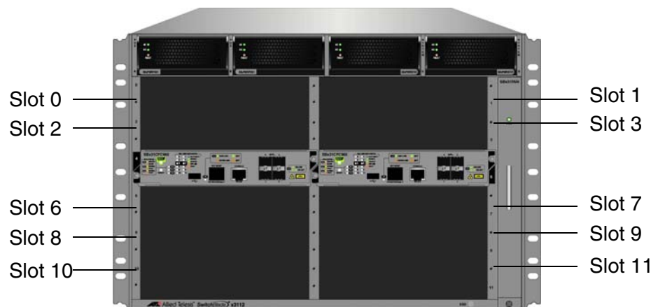
Figure 89. Slots 0 to 3 and 6 to 11 for the Ethernet Line Cards
