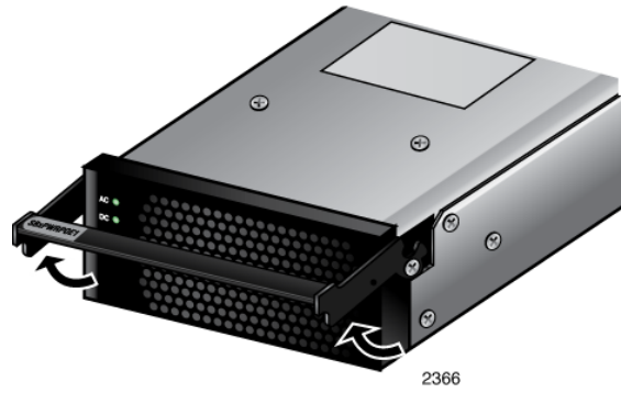
Figure 60. Raising the Handle on the AT-SBxPWRPOE1 Power Supply
