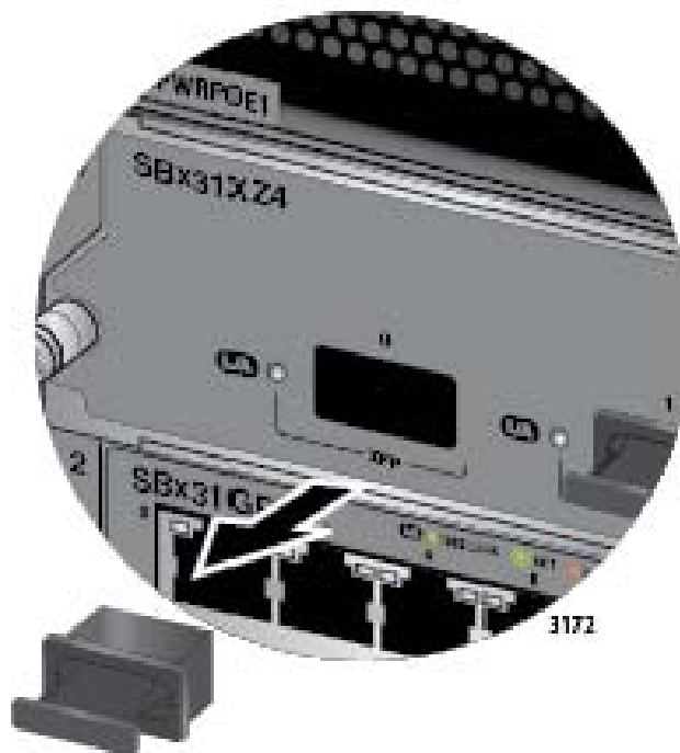
Figure 105. Removing the Dust Cover From an XFP Transceiver Slot on the AT-SBx31XZ4 Line Card
