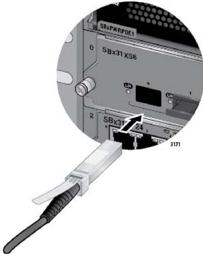
Figure 104. Installing the AT-SP10TW Cable in the AT-SBx31XS6 Line Card
