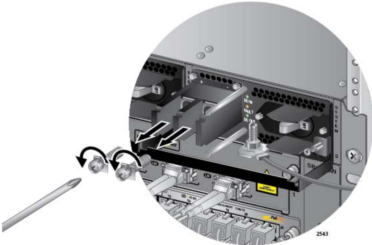
Figure 145. Removing the Terminal Screws
