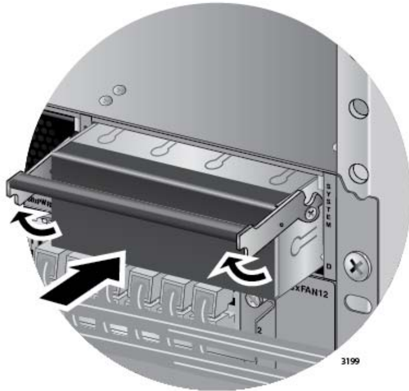
Figure 170. Installing a Blank Power Supply Slot Cover
