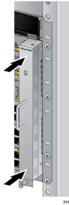
Figure 196. Securing the AT-SBxFAN12 Fan Module on the Backplane Connector
