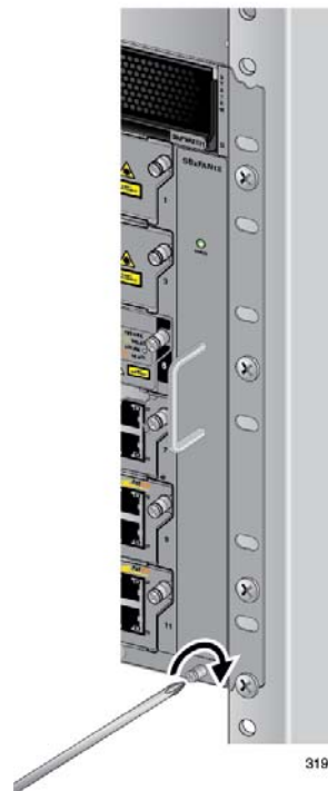
Figure 197. Tightening the Screw on the AT-SBxFAN12 Fan Module
