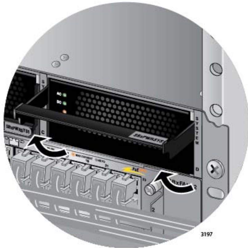
Figure 168. Lifting the Locking Handle on the Power Supply
