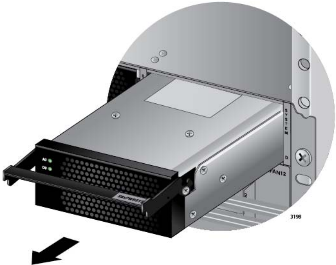
Figure 169. Removing the Power Supply from the Chassis
