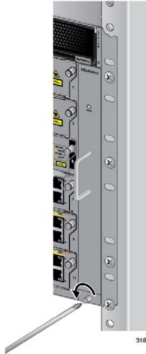
Figure 191. Loosening the Screw on the AT-SBxFAN12 Fan Module
