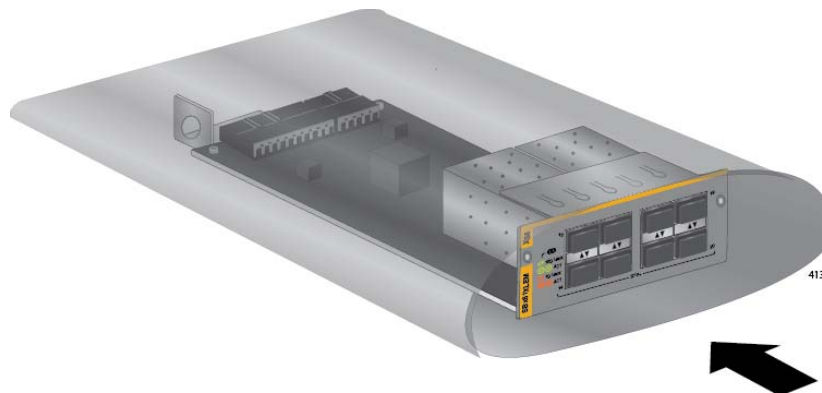
Figure 187. Storing the Expansion Module in an Anti-static Bag
