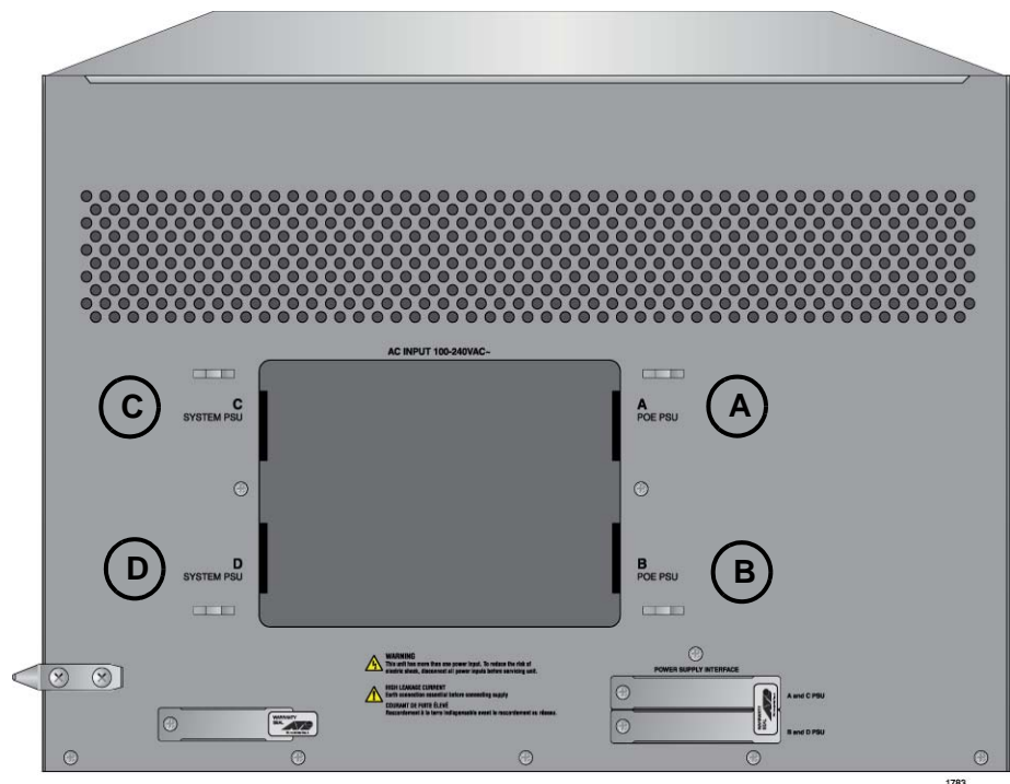
Figure 117. AC Sockets on the AT-SBx3112 Chassis Rear Panel
