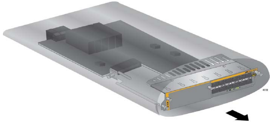
Figure 78. Removing the AT-SBx81XLEM Line Card from the Anti-static Bag
