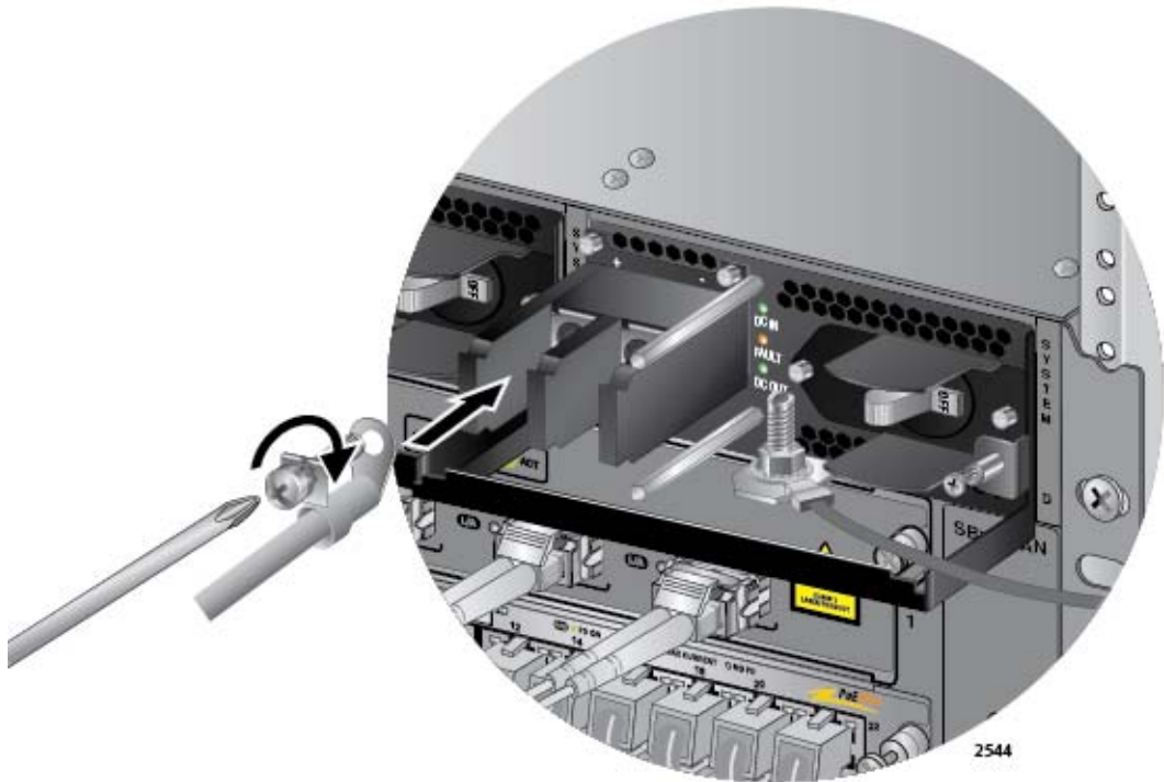
Figure 146. Connecting the Positive (+) Power Wire with a Right Angle Terminal
