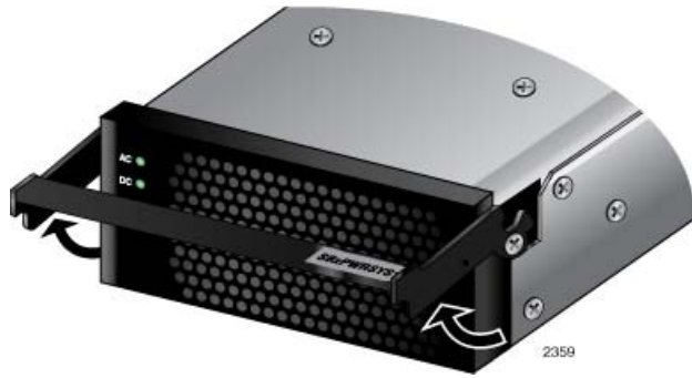
Figure 55. Raising the Handle on the Power Supply
