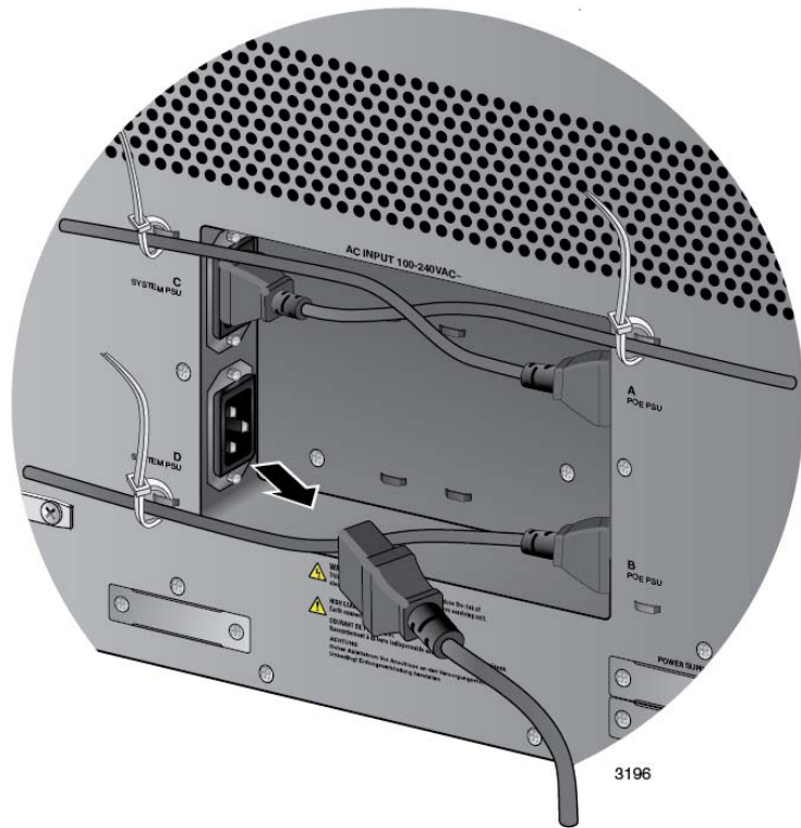
Figure 167. Disconnecting the AC Power Cord from the AC Socket on the Back Panel
