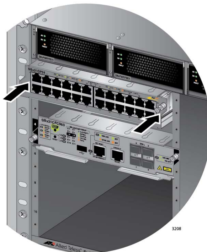
Figure 92. Seating an Ethernet Line Card on the Backplane Connector
