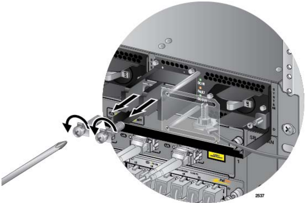
Figure 137. Removing the Terminal Screws
