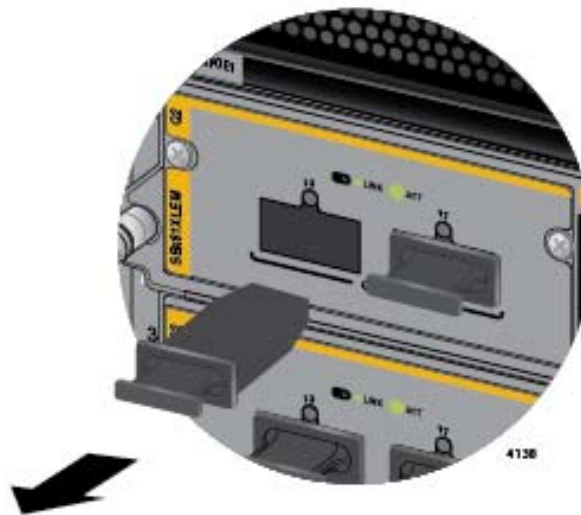
Figure 110. Removing the Dust Cover from a Transceiver Slot on the AT-SBx81XLEM/Q2 Expansion Module
