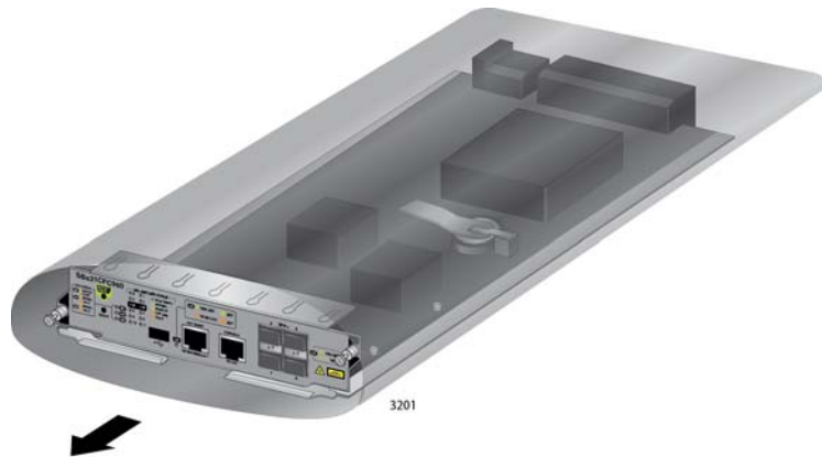
Figure 72. Removing the AT-SBx31CFC960 Controller Fabric Card from the Anti-static Bag
