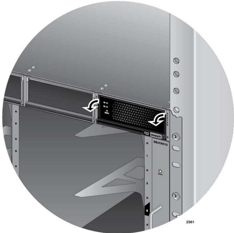
Figure 57. Lowering the Handle on the AT-SBxPWRSYS1 or AT-SBxPWRSYS2 AC Power Supply
