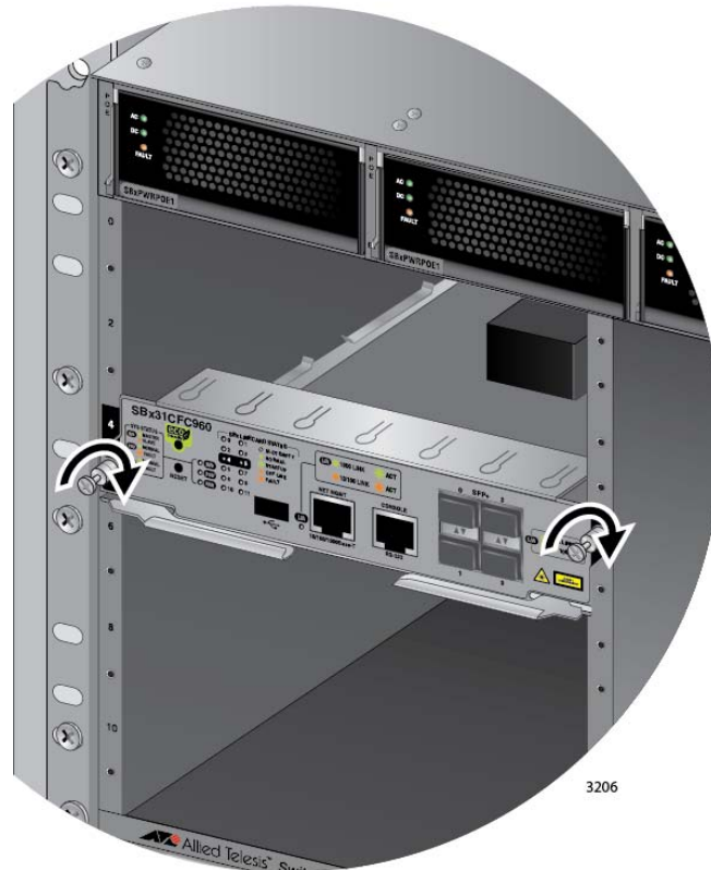
Figure 77. Tightening the Thumb Screws on the AT-SBx31CFC960 Card
