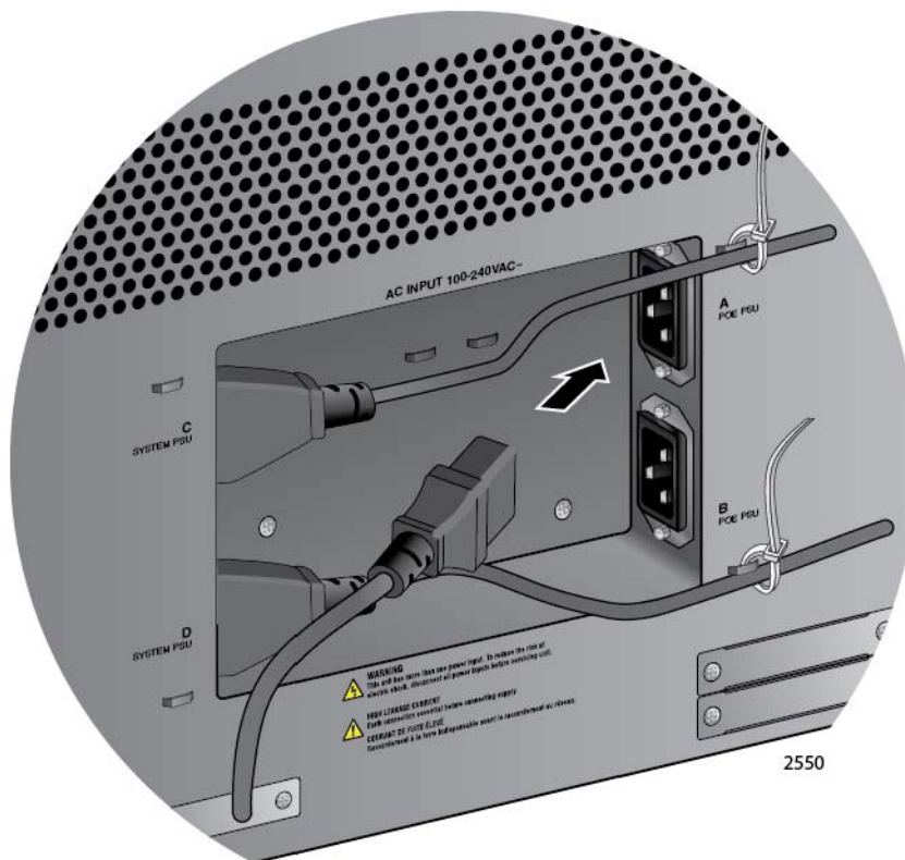
Figure 120. Connecting the AC Power Cord for the AT-SBxPWRPOE1 Power Supply
