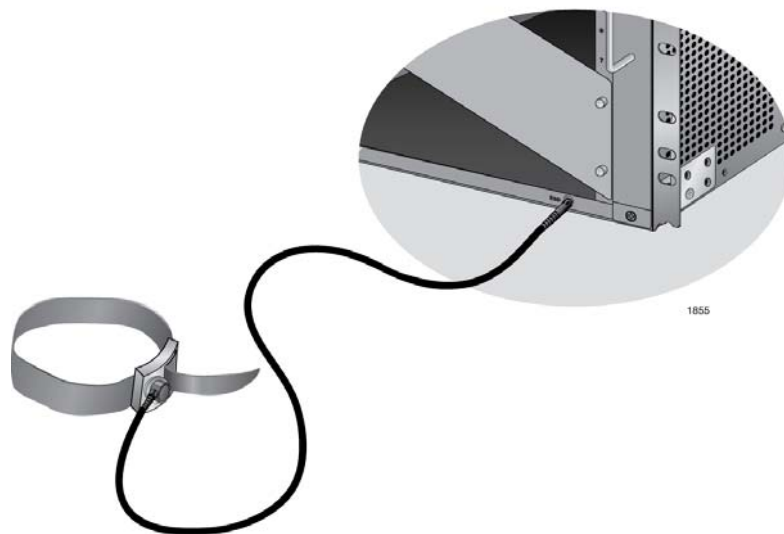
Figure 51. ESD Socket and Wrist Strap
