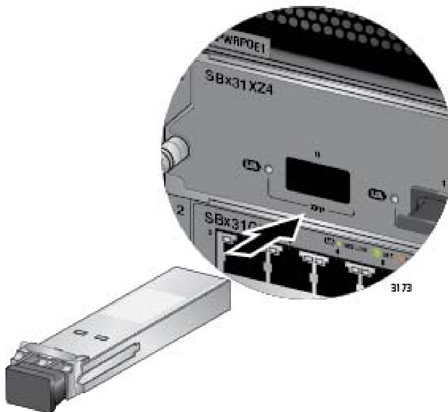
Figure 107. Installing an XFP Transceiver in the AT-SBx31XZ4 Line Card
