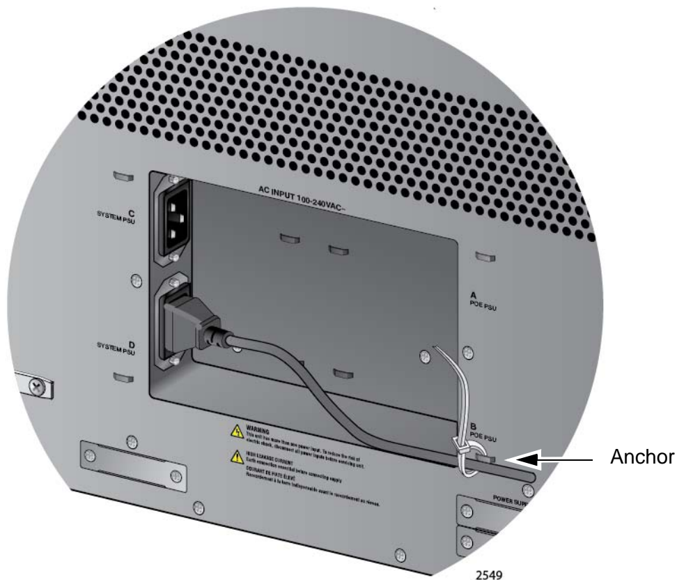
Figure 119. Securing the Power Cord for the AT-SBxPWRSYS1 or AT-SBxPWRSYS2 AC System Power Supply to an Anchor
