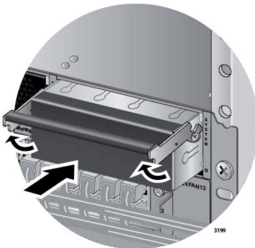
Figure 157. Installing a Blank Power Supply Slot Cover
