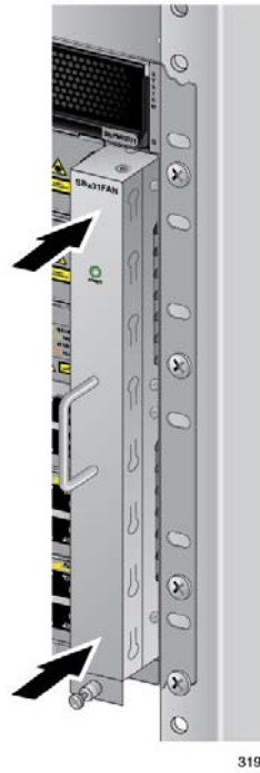
Figure 175. Securing the AT-SBx31FAN12 Fan Module on the Backplane Connector
