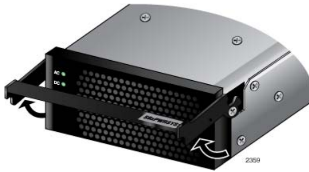
Figure 50. Raising the Handle on the Power Supply
