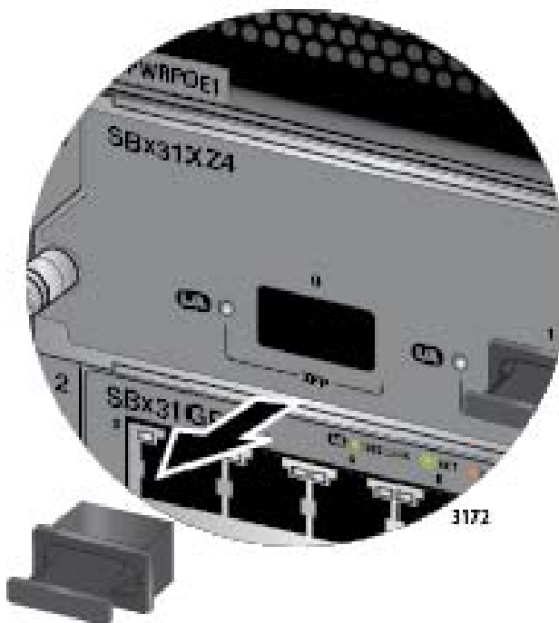
Figure 99. Removing the Dust Cover From an XFP Slot on the AT-SBx31XZ4 Line Card
