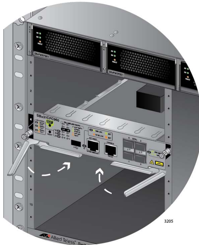
Figure 71. Closing the Locking Levers on the AT-SBx31CFC960 Controller Fabric Card
