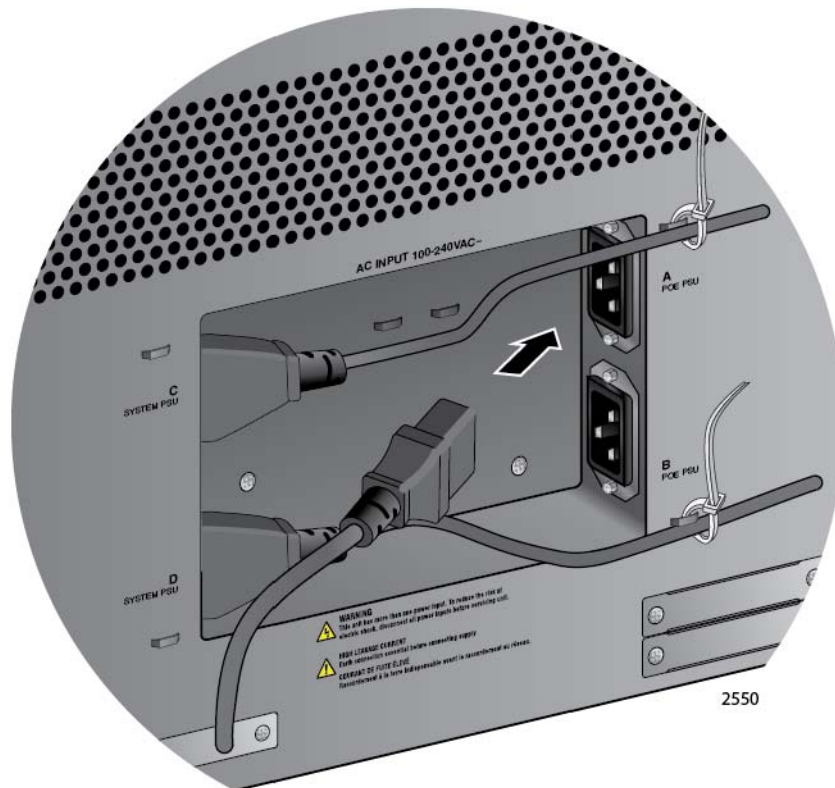
Figure 112. Connecting the AC Power Cord for the AT-SBxPWRPOE1 Power Supply
