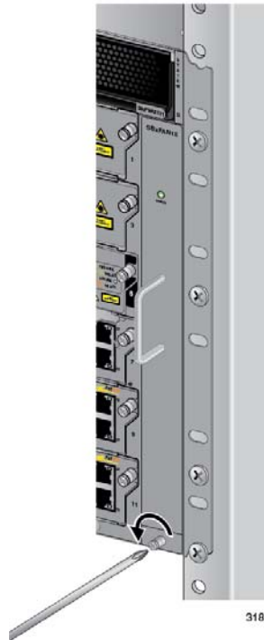
Figure 170. Loosening the Screw on the AT-SBxFAN12 Fan Module
