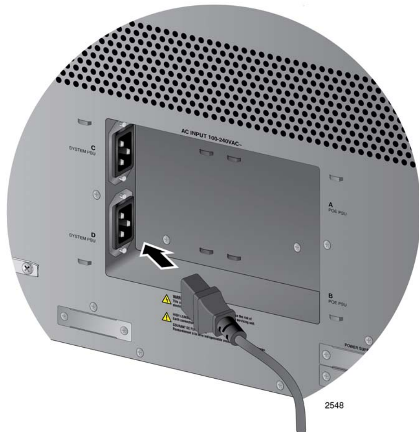
Figure 110. Connecting the AC Power Cord for the AT-SBxPWRSYS1 or AT-SBxPWRSYS2 AC System Power Supply
