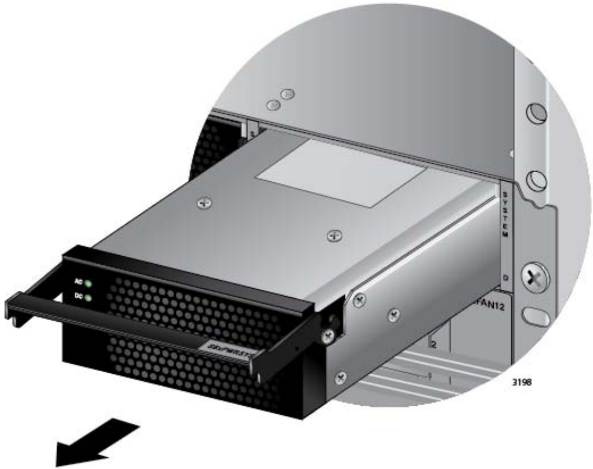
Figure 156. Removing the Power Supply from the Chassis
