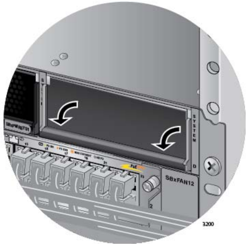
Figure 158. Lowering the Locking Handle on the Power Supply Slot Cover
