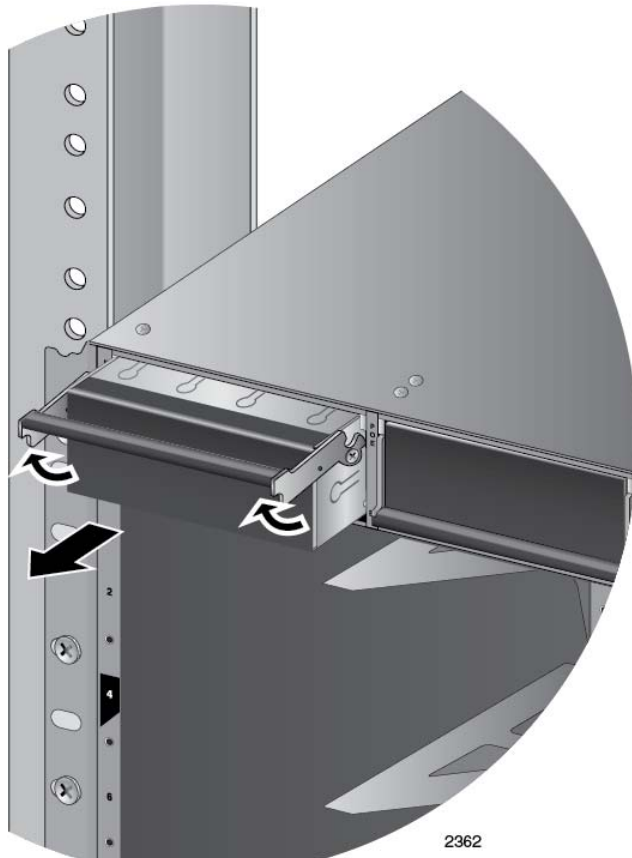
Figure 53. Removing the Blank Slot Cover from Power Supply Slot A
