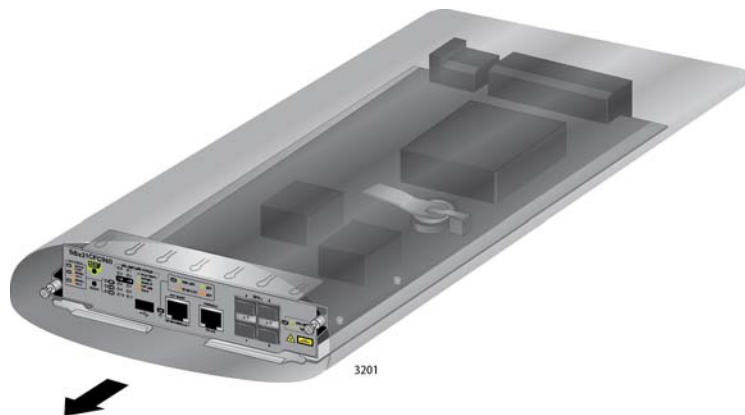
Figure 67. Removing the AT-SBx31CFC960 Controller Fabric Card from the Anti-static Bag
