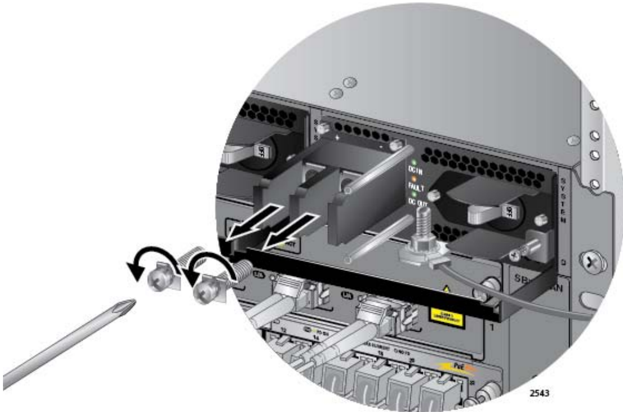
Figure 137. Removing the Terminal Screws
