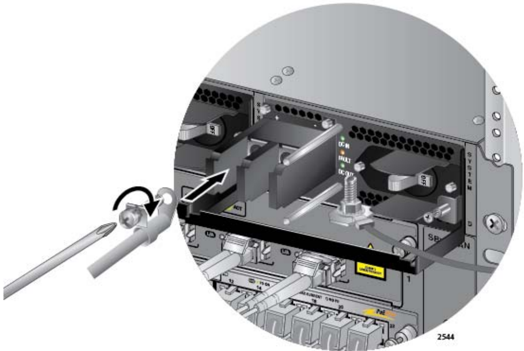
Figure 138. Connecting the Positive (+) Power Wire with a Right Angle Terminal
