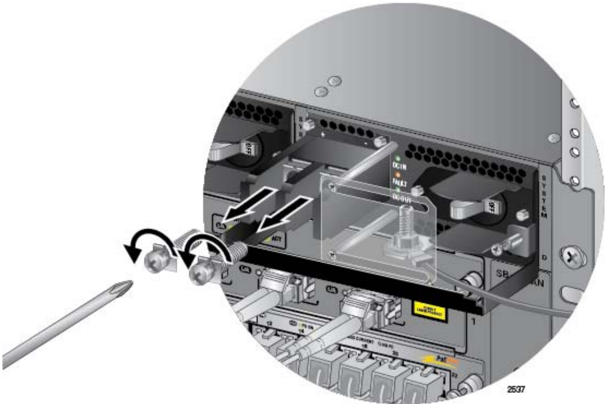
Figure 129. Removing the Terminal Screws
