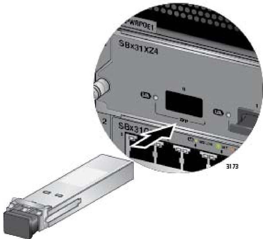
Figure 101. Installing an XFP Transceiver in the AT-SBx31XZ4 Line Card
