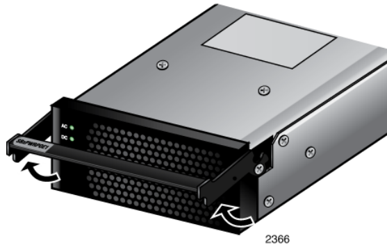
Figure 55. Raising the Handle on the AT-SBxPWRPOE1 Power Supply
