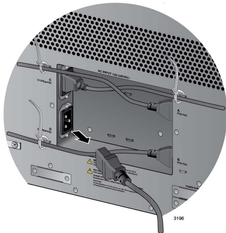
Figure 154. Disconnecting the AC Power Cord from the AC Socket on the Back Panel
