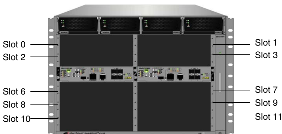
Figure 73. Slots 0 to 3 and 6 to 11 for the Ethernet Line Cards
