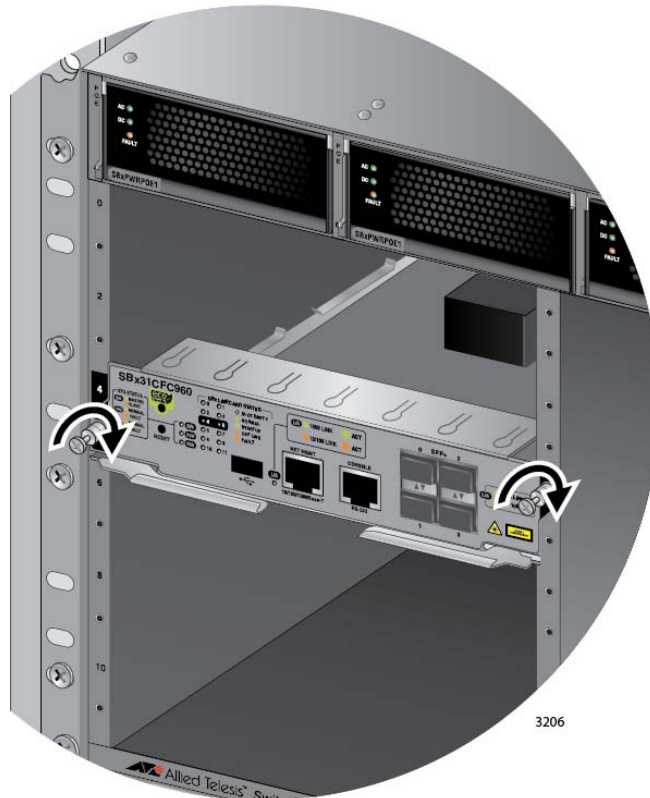
Figure 72. Tightening the Thumb Screws on the AT-SBx31CFC960 Card
