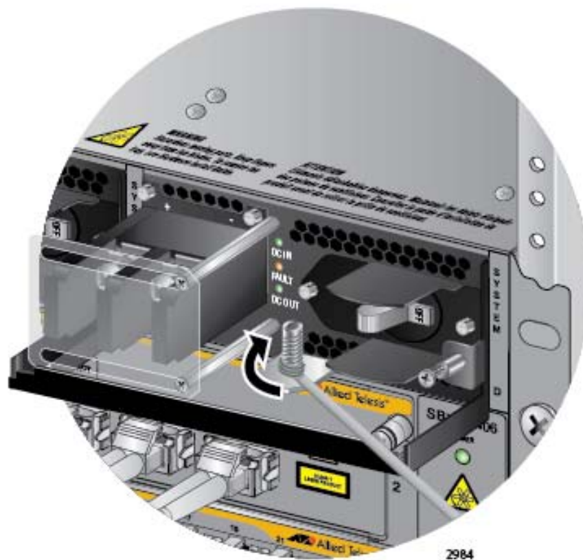
Figure 120. Attaching the Bare Grounding Wire to the Grounding Post
