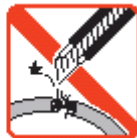
Figure 9: Do not damage power cable
