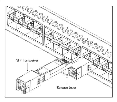
Slide the transceiver into the SFP socket, and firmly press it until it engages. To remove it, first release it by gently pulling the release lever, and then pull the transceiver out of the socket. **Never** force a transceiver into or out of a socket.
