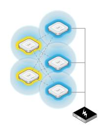
Allied Telesis AWC Smart Connect (AWC-SC) is an effortless wireless network expansion with no added wires. Just register the new AP, plug in the power and it's ready.
