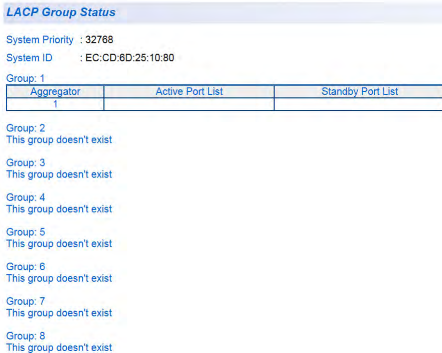
Figure 38. LACP Group Status Page with No Cables Connected
