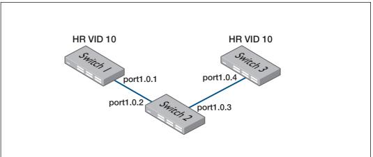
Without GVRP, you would have to manually add the HRVLAN 10 to Switch 2. But with GVRP, the VLAN is added automatically. Here is how GVRP resolves this example.
