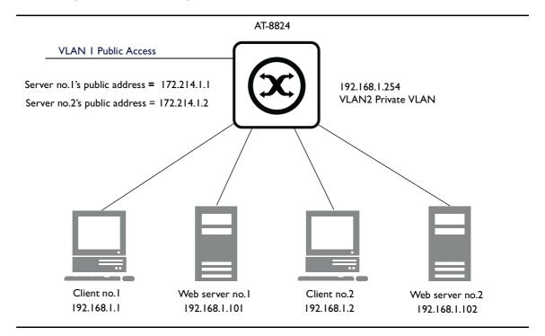
I. Create a private VLAN for access-level /shared users'. Private VLANs ensure that the ports of this VLAN cannot send traffic directly to each other. They must use an uplink or be layer 3 routed through the firewall:
