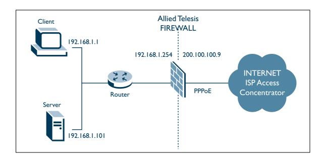
The whole subnet 200.100.100.8/255.255.255.248 has been allocated to the site where the Allied Telesis firewall is located. So the ISP will route ANY addresses in that subnet to the Allied Telesis firewall.
