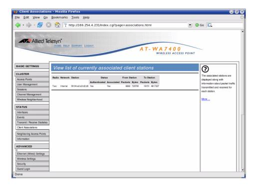
Notice that in the above picture we have changed the GUI view to a different Access Point (169.254.4.231). This is because the client was actually in an area best covered by the second Access Point. When this happens, the first Access Point (169.254.4.230) does not have a record of a client associated with another Access Point even though, by default, the two Access Points are in a cluster.
