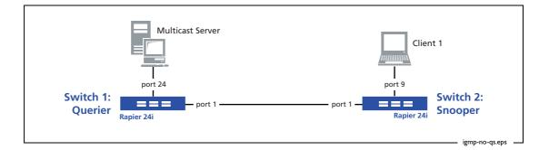
The example considers what happens when a port comes up. When the port was down, the client stopped receiving multicasts, because there was no backup route available. The example shows how the network recovers. The multicast group is 224.12.13.14.
