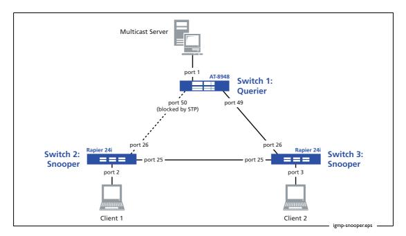
The network contains a Windows 2000 workstation that regularly sends SVRLOC messages (an IGMP Membership Report for 224.0.1.22). This group gets added to the list of groups in vlan100 on switch 1, as shown in the following output of the **show ip igmp** command.
