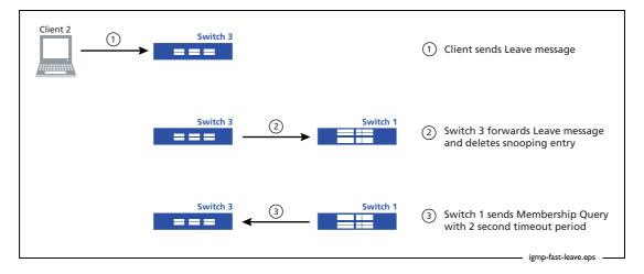
The result of this is that switch 3 adds the group back into its snooping table (with the same timeout as the IGMP Querier) but has no ports interested in receiving the group. Because Fast Leave is enabled on port 3, that port was removed from the group as soon as switch 3 received the Leave message.
