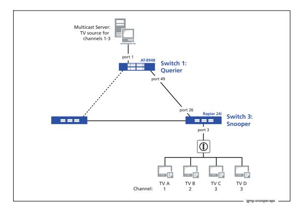
In this situation, you need to use fast leave in **multiple host mode**. In multiple host mode, the Snooper tracks which clients are joined to a given IP multicast group on a given port. The Snooper shuts off the multicast group to that port as soon as the **last** client leaves the group on the port.
