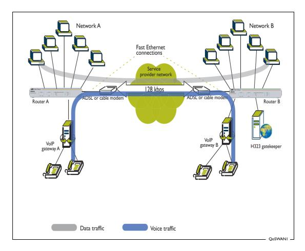
Potentially large volumes of data are being exchanged between computer networks A and B, whilst Voice over IP (VoIP) calls are also being transported across the WAN link.
