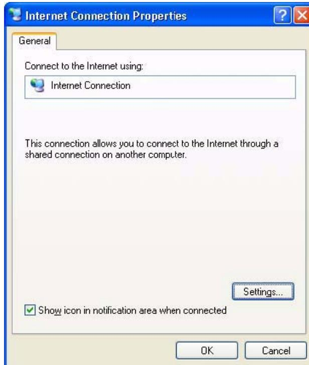
2. Click the **Settings** button. This opens the **Advanced Settings** window. The following screen capture shows that two port mappings have been added by the Windows Messenger. This is the NAT Traversal functionality—port mappings are automatically added without user configuration.
