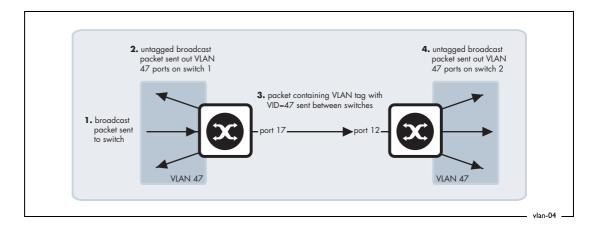
The tag makes it very easy for the second switch to know what to do with the packet, because the tag marks this packet as belonging to VLAN 47, and switch 2 knows exactly what it should do with packets that belong to VLAN 47.
