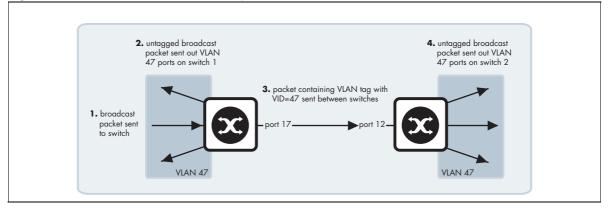
The tag makes it very easy for the second switch to know what to do with the packet, because the tag marks this packet as belonging to VLAN 47, and switch 2 knows exactly what it should do with packets that belong to VLAN 47.
