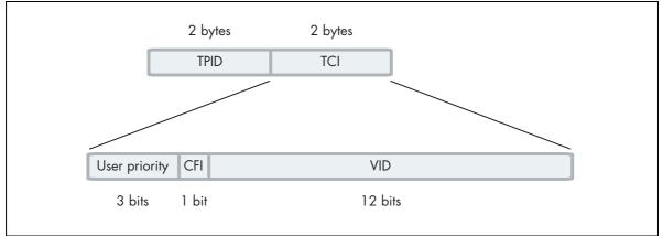
**TPID** is the tag protocol identifier, which indicates that a tag header is following and contains the user priority, Canonical Format Indicator (CFI), and the VLAN ID.
