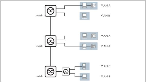
Instead of the LANs corresponding to physical areas divided from each other by routers, there are virtual LANs distributed across the network. For example, all the devices in the various areas labeled 'LAN A' all belong to a single virtual LAN—i.e. a single broadcast domain.
