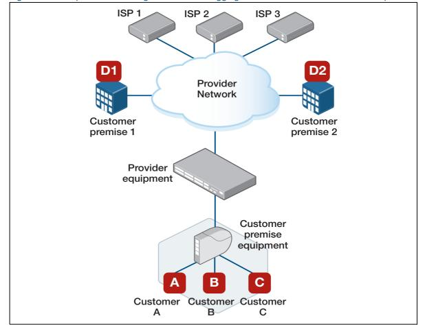
Figure 11: Example network using VLAN double-tagging and VLAN translation on the same port
