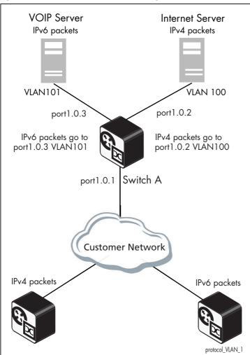
Switch A has the following configuration to enable protocol based VLAN classification:
