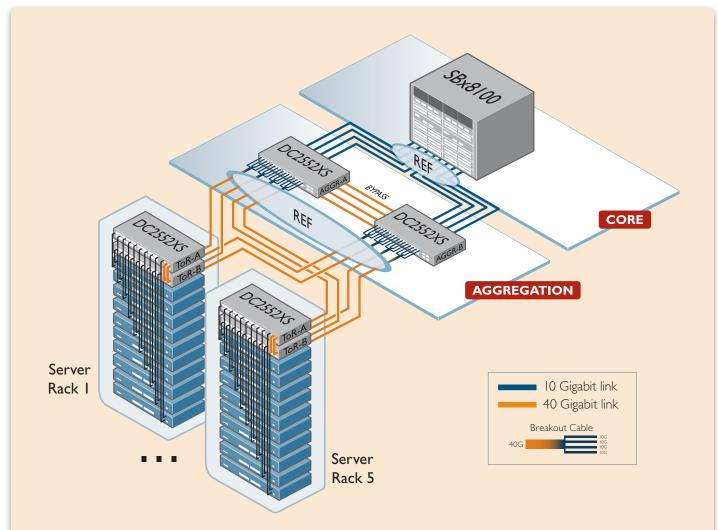
This network configuration enables server and storage to communicate within two layers, securing the low-latency and high-speed connection. The bypass supports up to 160Gbps for aggregation mode or 80Gbps for ToR mode.
