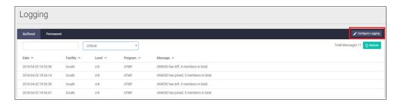
In the **Logging Configuration** page, you can create filters to manage which logs are stored on the device and also set up a Syslog server(s) for remote log storage.
