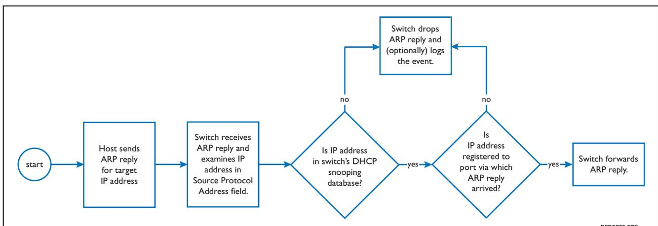
Therefore, ARP security makes it impossible for a host to poison the ARP caches of other hosts, because the switch only forwards ARP packets that have genuine information in the Source Protocol Address field.
