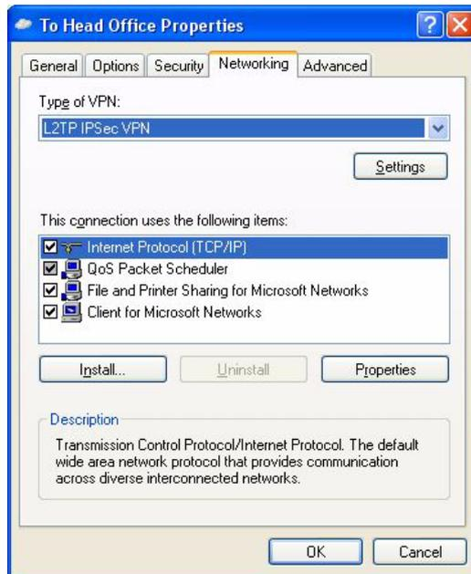
7. Click **OK**. This completes the configuration of the L2TP client. To connect to the office, click **Connect**. Note that the connection will fail if the router has not yet been configured.
