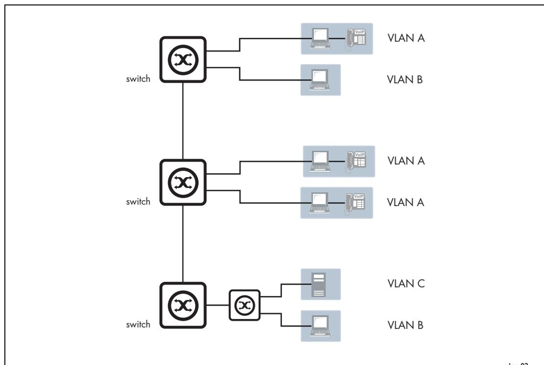
So, instead of the LANs corresponding to physical areas divided from each other by routers, there are virtual LANs distributed across the network. For example, all the devices in the various areas labelled “VLAN A” all belong to a single virtual LAN—i.e. a single broadcast domain.
