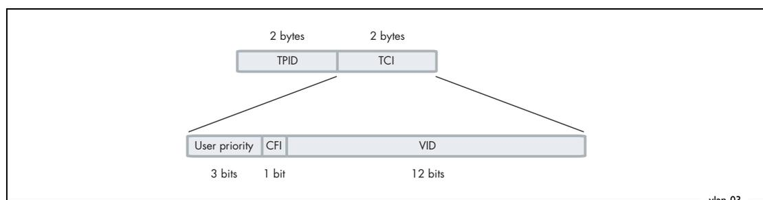
TPID is the tag protocol identifier, which indicates that a tag header is following and contains the user priority, canonical format indicator (CFI), and the VLAN ID.
