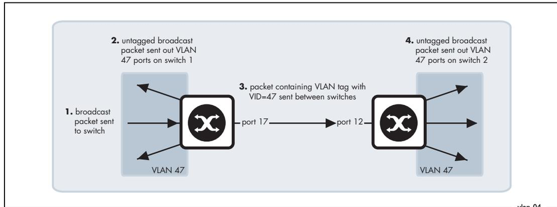
The tag makes it very easy for the second switch to know what to do with the packet, because the tag marks this packet as belonging to VLAN 47, and switch 2 knows exactly what it should do with packets that belong to VLAN 47.
