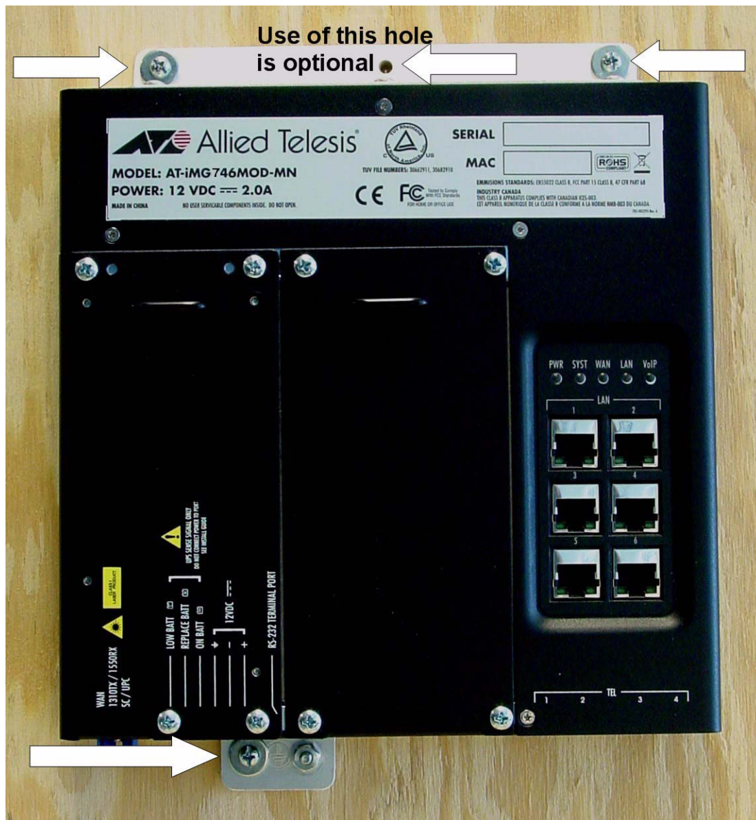
Figure 20. Securing the Gateway to the Mounting Surface
