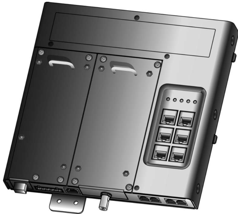
Figure 1. The AT-iMG746MOD Electronics Unit (with Gig BiDi WAN Module)
