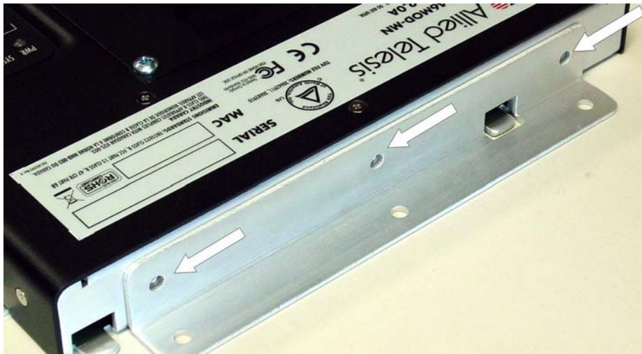
Figure 19. Attaching the Wall Mount Bracket to the iMGxx6MOD (Mounting Holes)
