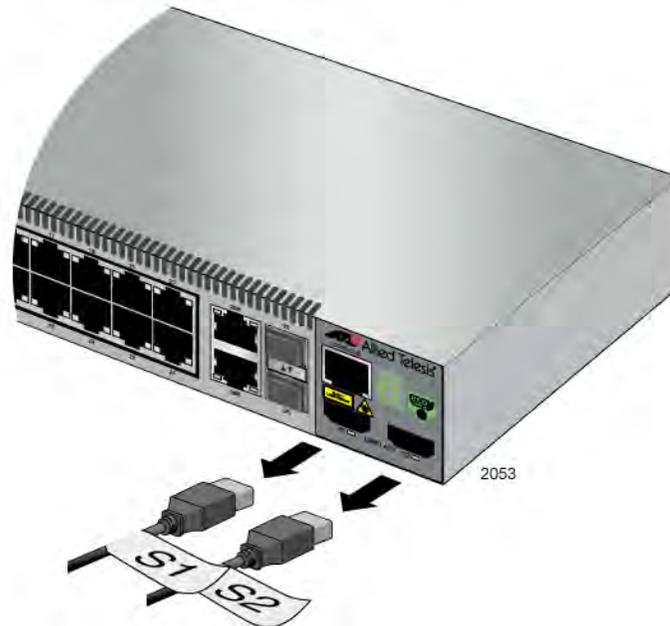
Figure 57. Removing the Stacking Cables
