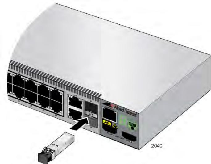
Figure 46. Installing an SFP Transceiver
