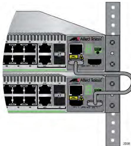
Figure 34. Connecting the Stacking Cable
