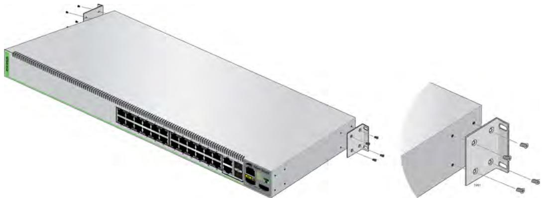
Figure 24. Attaching the Brackets to Install the Switch in an Equipment Rack (Continued)
