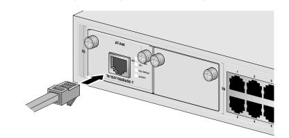
11. Make sure the LINK LED on the front of the expansion module is steady green. (A 1000Base port may require from five to ten seconds to initially establish a link with an end node.)
