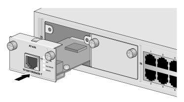
8. Secure the expansion module to the switch by using a Phillips screwdriver to tighten the installation screws found on the expansion module faceplate.
