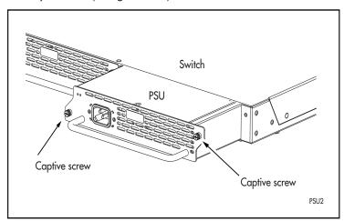
Slowly and carefully slide the PSU or FOM out of the bay. Support the device from underneath as you remove it to prevent it from falling.
