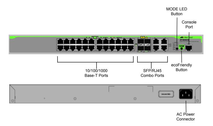
Figure 3. AT-9000/28 Switch Front and Rear Panels
