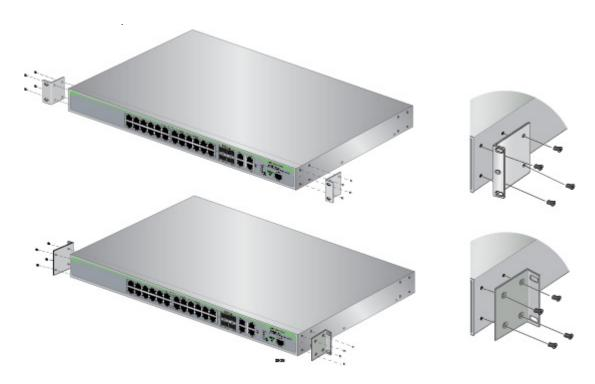
Figure 14. Attaching Brackets for Rack Mounting
