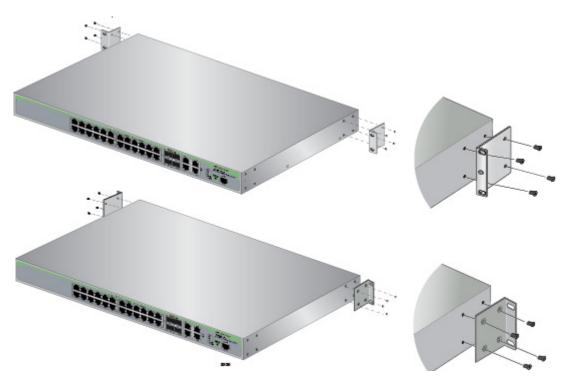
Figure 15. Attaching Brackets for Rack Mounting (Continued)
