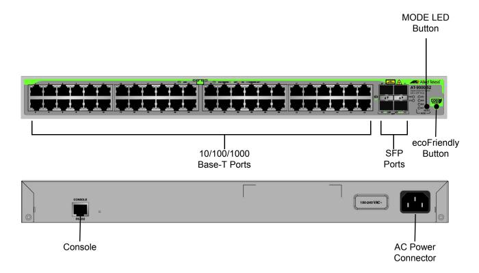
Figure 6. AT-9000/52 Switch Front and Rear Panels
