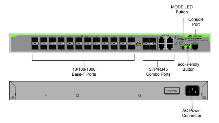
Figure 5. AT-9000/28SP Switch Front and Rear Panels
