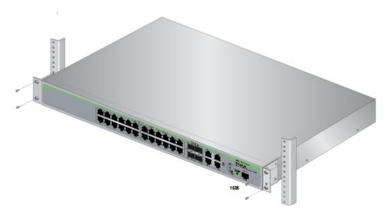
Figure 16. Mounting the Switch in a Rack
