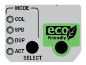
Figure 10. Front Panel MODE LED SELECT Button and LEDs
