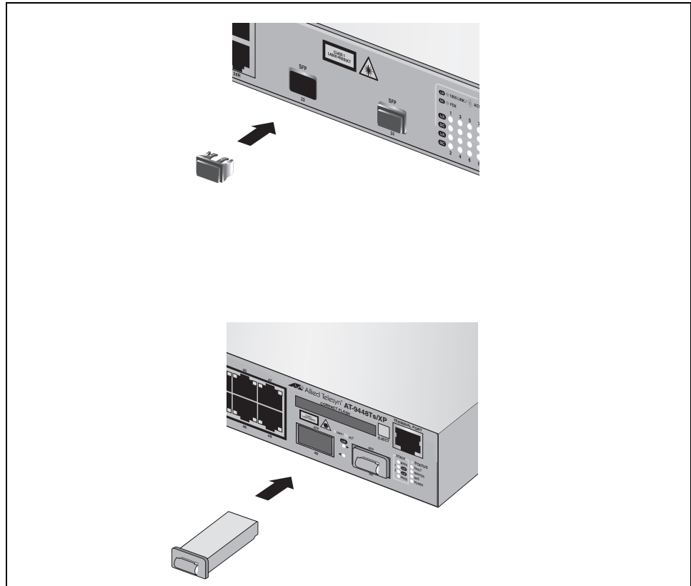
Figure 41. Installing the Dust Covers in the SFP and XFP Slots
