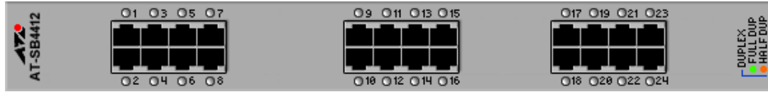
24-Port (RJ-45) 10BASE-T/100BASE-TX/1000BASE-T Gigabit Ethernet Line Card
