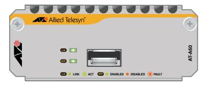
The following LEDs report operations and faults on the AT-A60.
