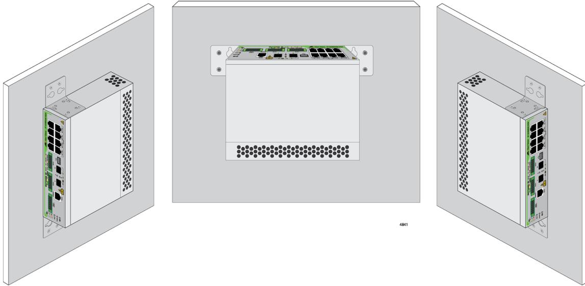
Figure 48. Positioning the GS980EM/10H or GS980EM/11PT Switch on the Wall
