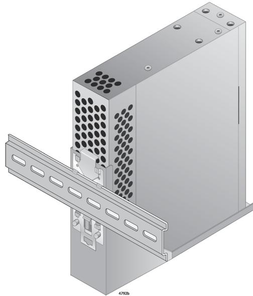
Figure 47. Verifying the DIN Rail Installation
