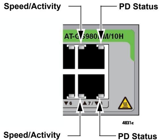
Figure 2. LEDs for Ports 1 to 8 on the GS980EM/10H Switch.
