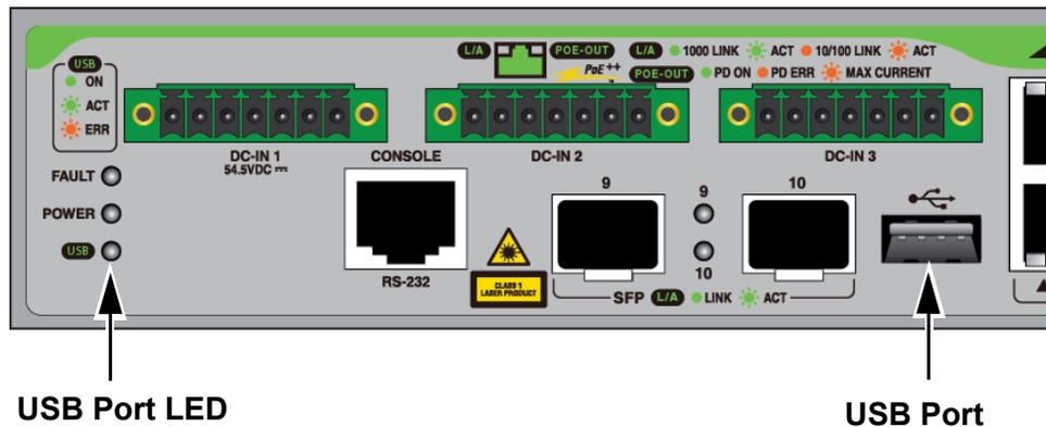
Figure 5. GS980EM/10H USB Port and LED
