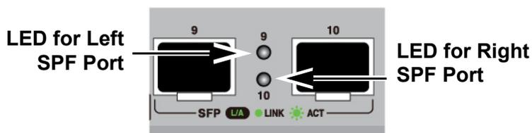
Figure 11. SFP Transceiver Ports LEDs
