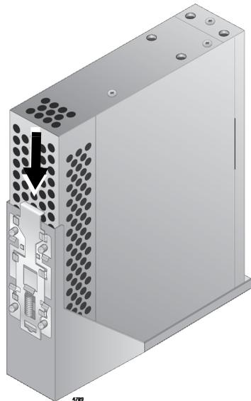
Figure 45. Pressing Down on the Spring-Loaded Lever
