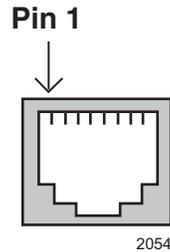
Figure 75. RJ-45 Socket Pin Layout (Front View)
