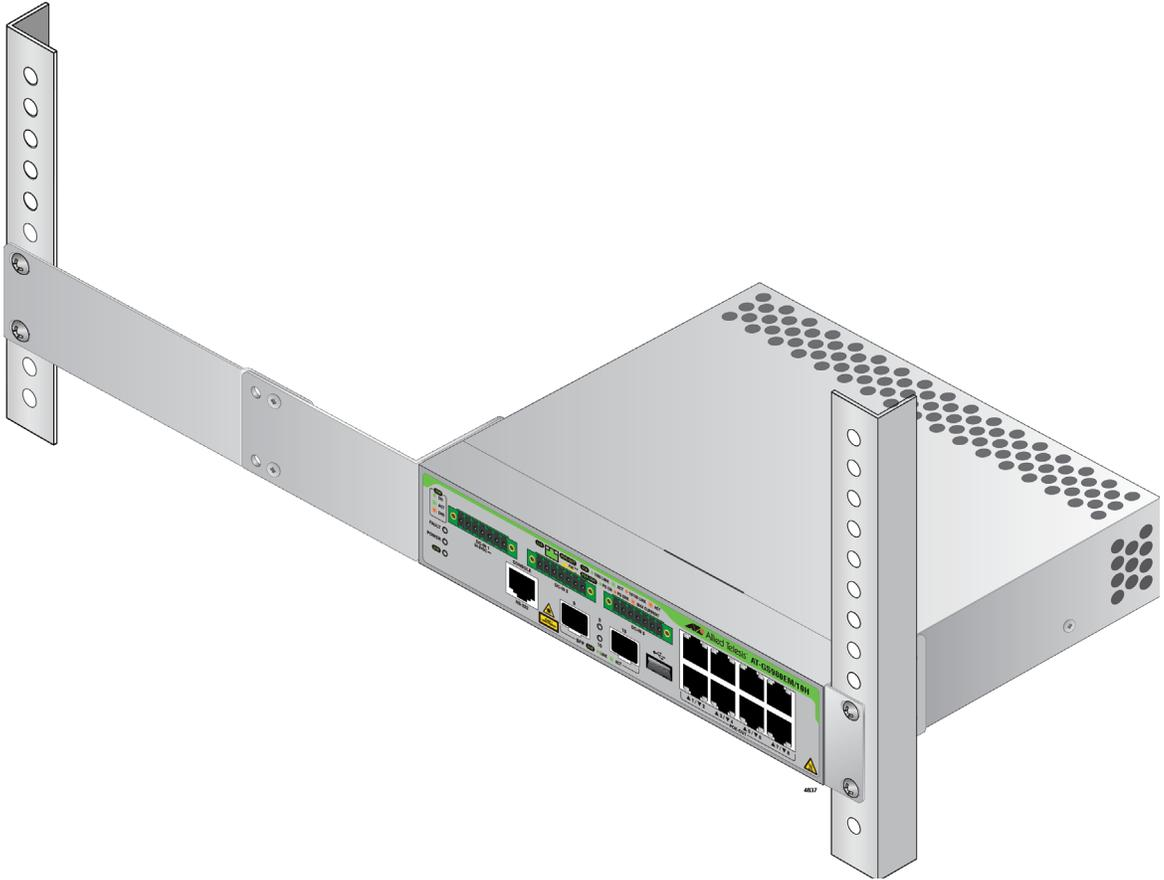
Figure 33. Device Secured in an Equipment Rack
