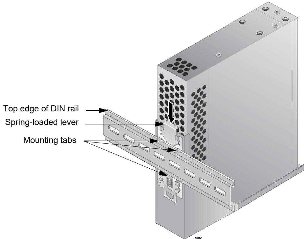
Figure 46. Installing the Device on a DIN Rail
