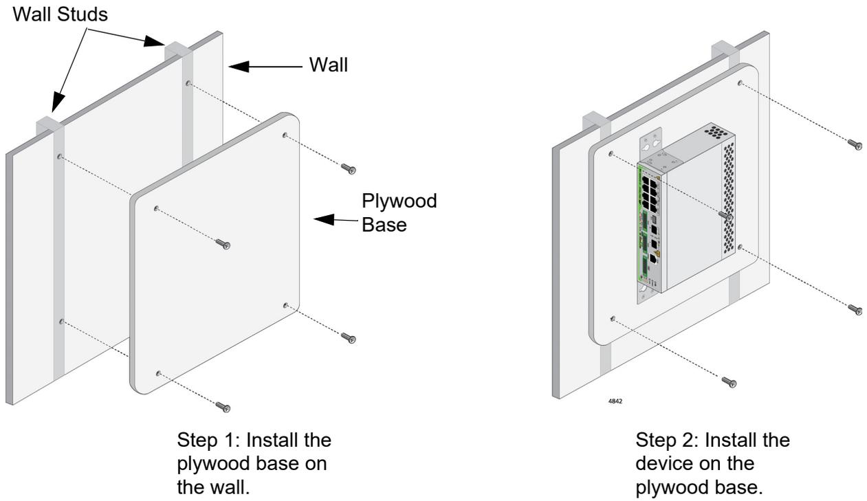
Figure 51. Steps to Installing the Device with a Plywood Base
