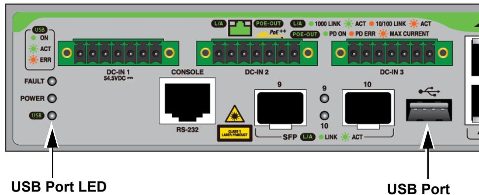
Figure 12. GS980EM/11PT USB Port and LED
