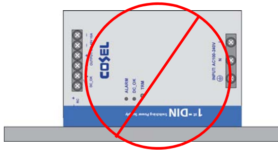
Figure 7. Unsupported Table, Desk, or Shelf Installation
