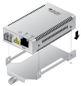
2. Tighten four screws to attach the carrier bracket and media converter.
