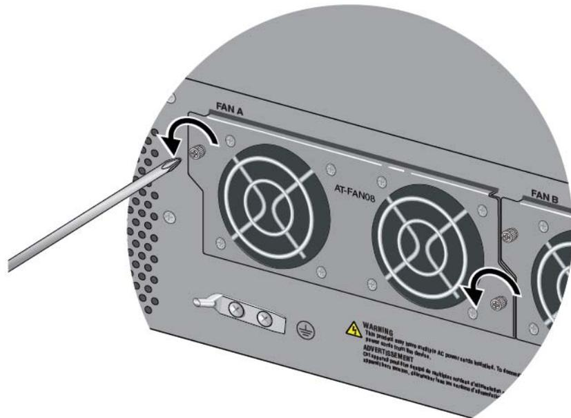
Figure 127. Loosening the Screws on the FAN08 Module
