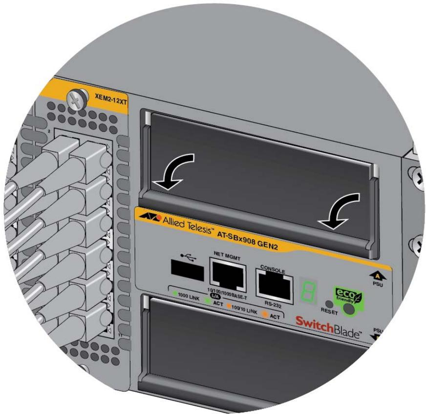
Figure 122. Lowering the Locking Handle on the Power Supply Slot Cover
