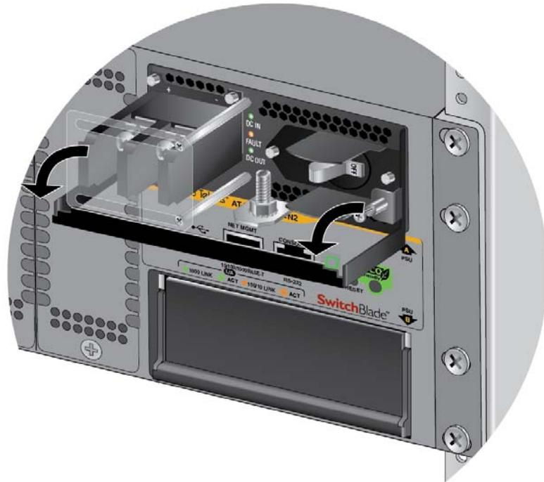
Figure 55. Lowering the Locking Handle on the SBxPWRSYS1-80 DC Power Supply
