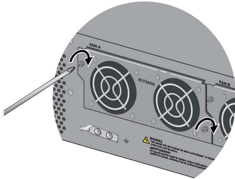
Figure 131. Tightening the Two Captive Screws on the FAN08 Module
