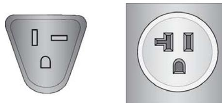
Figure 29. NEMA 5-20P Plug and Receptacle
