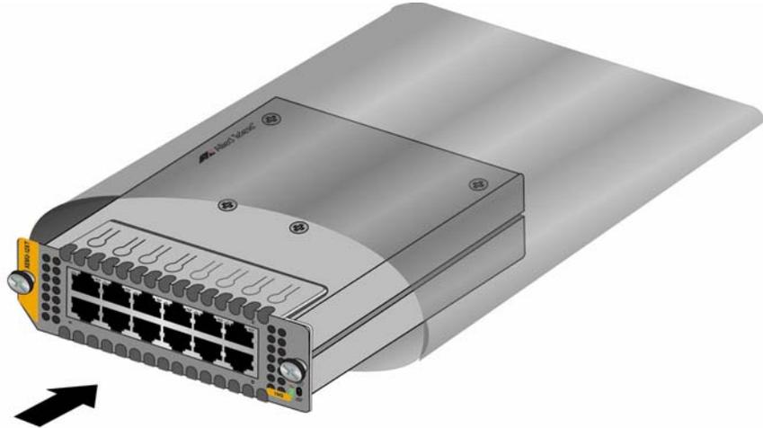
Figure 126. Placing the Ethernet Line Card in its Anti-static Bag
