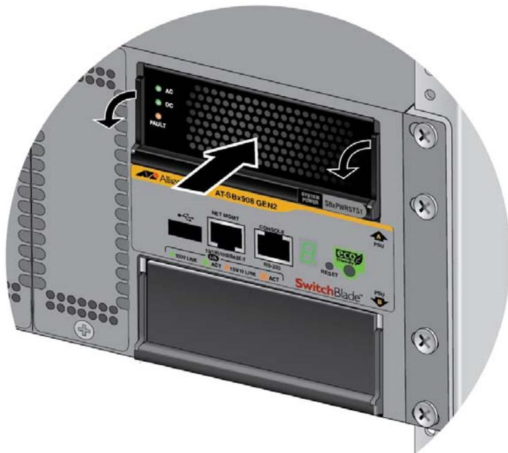
Figure 50. Lowering the Locking Handle on the SBxPWRSYS2 AC Power Supply
