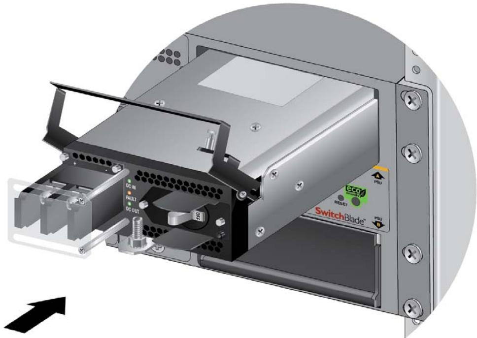
Figure 54. Inserting the SBxPWRSYS1-80 DC Power Supply
