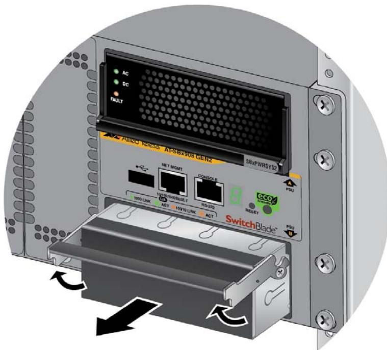
Figure 47. Removing the Blank Power Supply Panel from Power Supply Slot B
