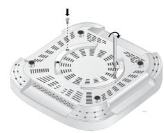
Align and insert the mounting bracket keyholes over the two screws installed in Step 1 and slide the bracket into the narrow part of the keyhole slots. Refer to the following figure.
