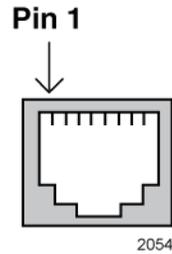
Figure 16. RJ-45 Socket Pin Layout (Front View)
