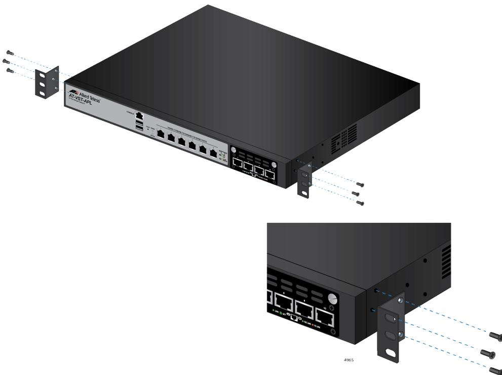
Figure 11. Attaching Brackets to the Vista Manager Appliance
