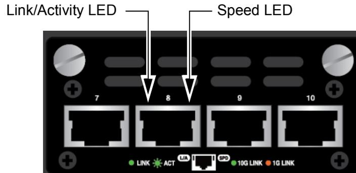
Figure 5. LEDs for the 1/10GBase-T Twisted Pair Ports
