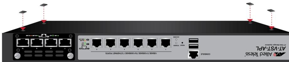
Figure 10. Attaching the Rubber Feet
