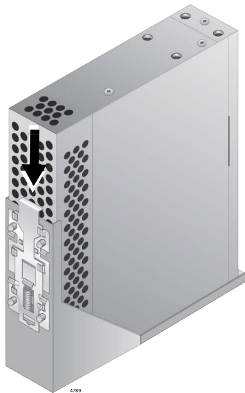
Figure 45. Pressing Down on the Spring-Loaded Lever
