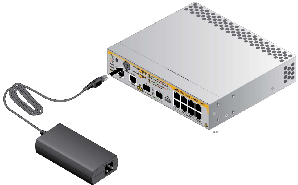
Figure 68. Connecting the PWR90ADP Power Adapter to the x320-11GPT Switch
