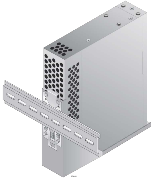
Figure 47. Verifying the DIN Rail Installation
