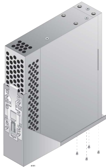
Figure 43. Screwing the Device to the DRMT-J03 DIN Chassis Bracket
