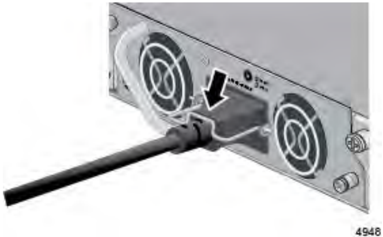
Figure 52. Plugging in the AC Power Cord to the Switch
