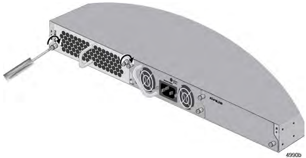
Figure 106. Tightening the Two Captive Screws on the FAN10 / FAN10R Module
