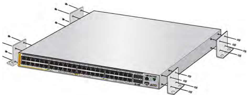
Figure 41. Installing Brackets on the Switch
