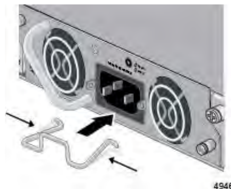
Figure 50. Installing the Power Cord Retaining Clip
