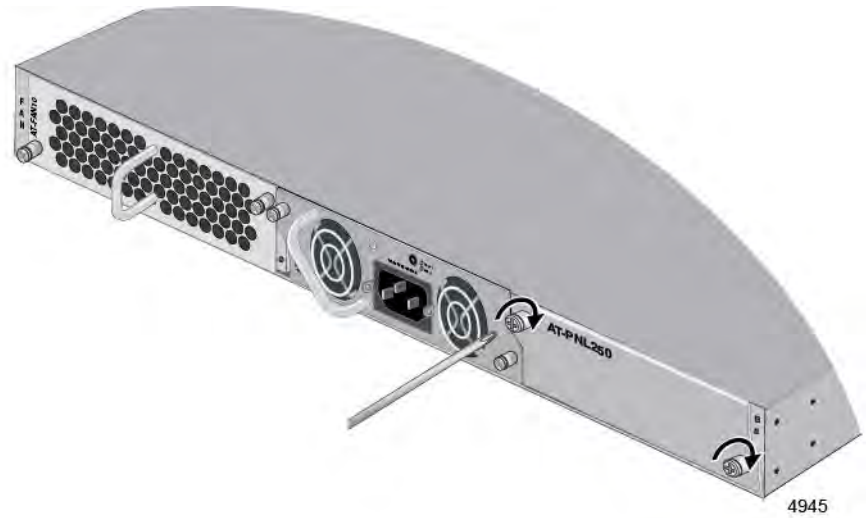
Figure 33. Tightening the Captive Screws on the Power Supply Blank Panel
