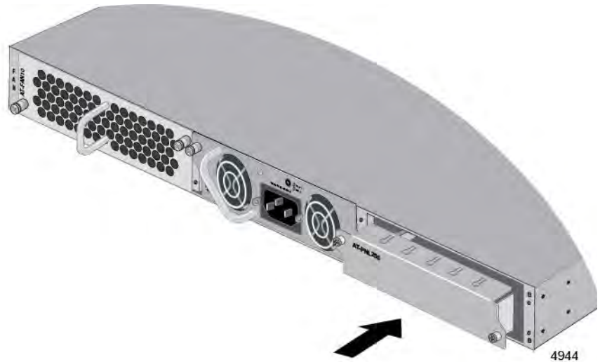
Figure 100. Installing a Blank Panel on a Power Supply Slot
