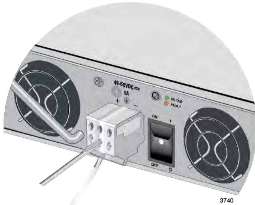
Figure 48. Connecting the Ground Wire to the DC Terminal Block
