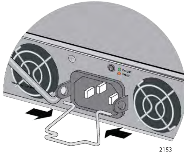
Figure 31. Installing the Power Cord Retaining Clip
