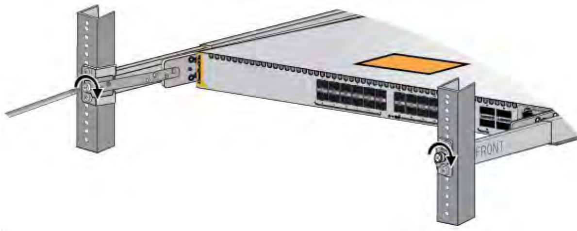
Figure 89. Tightening the Two Screws on the Fixed Brackets
