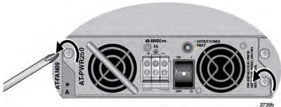
Figure 98. Loosening the Two Captive Screws
