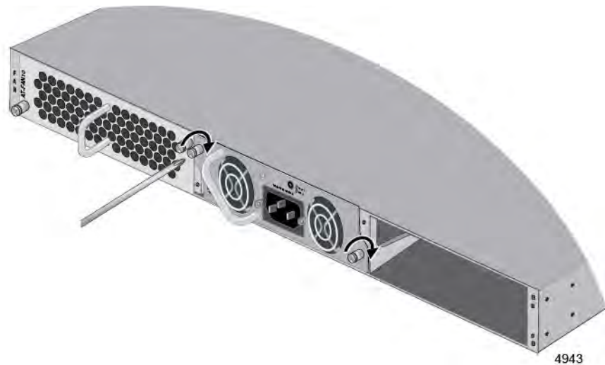
Figure 30. Tightening the Captive Screws on the Power Supply
