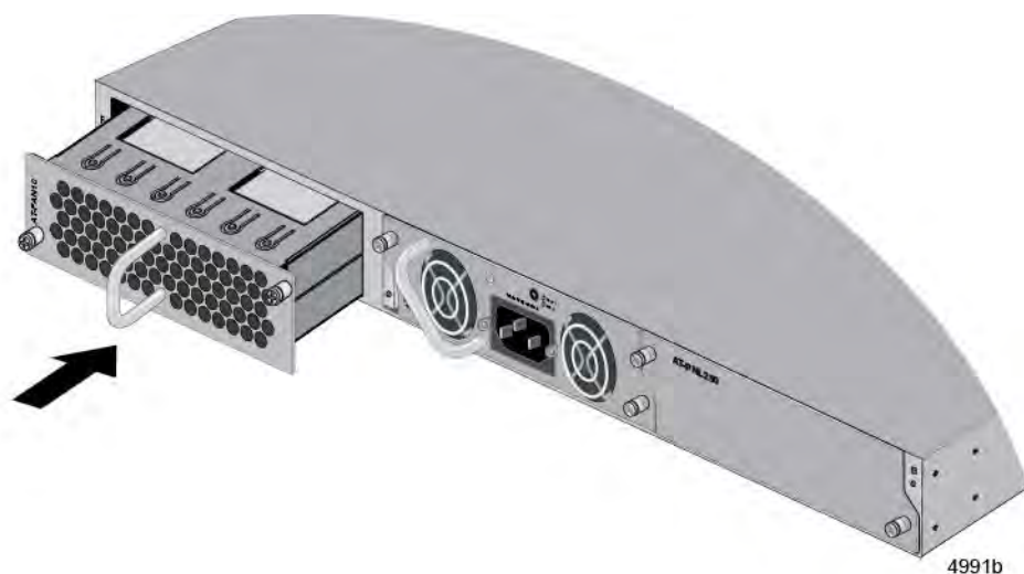
Figure 104. Aligning the FAN10 / FAN10R Module in the Switch Slot
