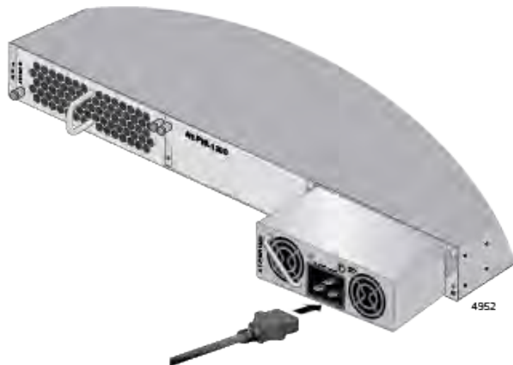
Figure 54. Connecting the AC Power Cord to the Switch
