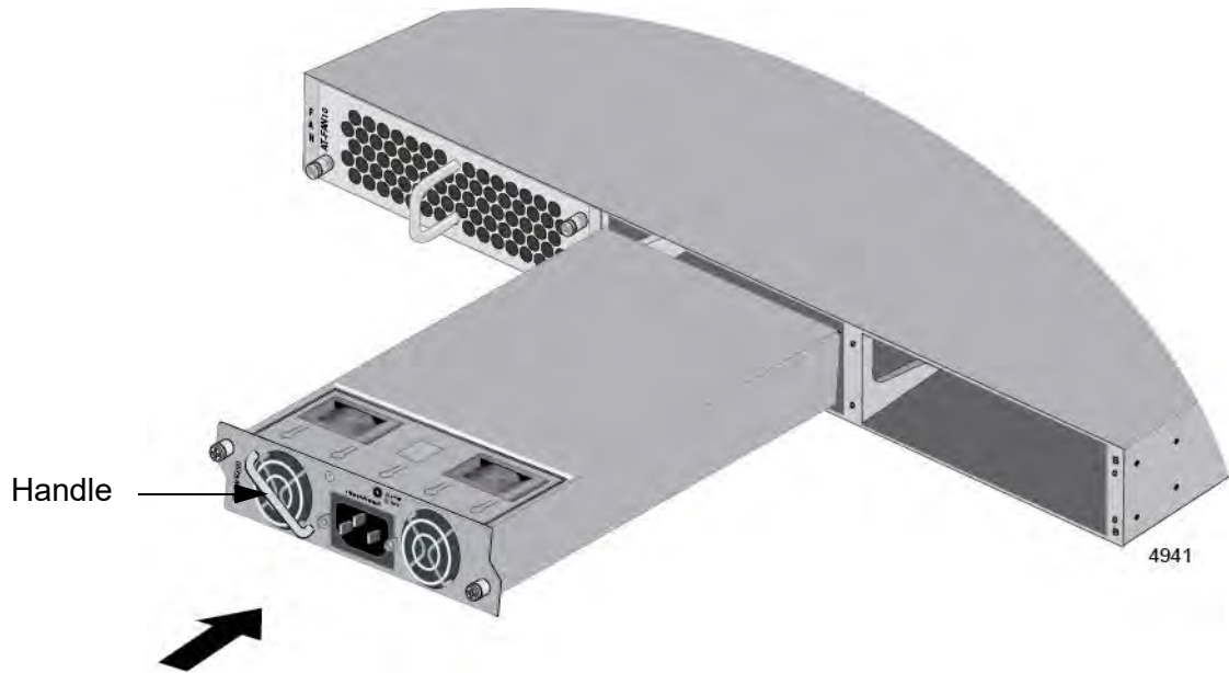
Figure 28. Installing a Power Supply
