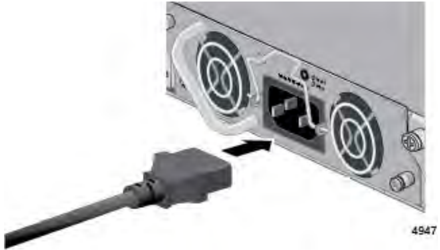
Figure 51. Connecting the AC Power Cord to the Switch
