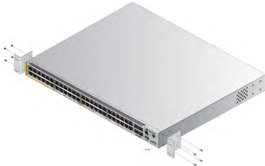
Figure 36. Example of Attaching the Brackets to the Switch
