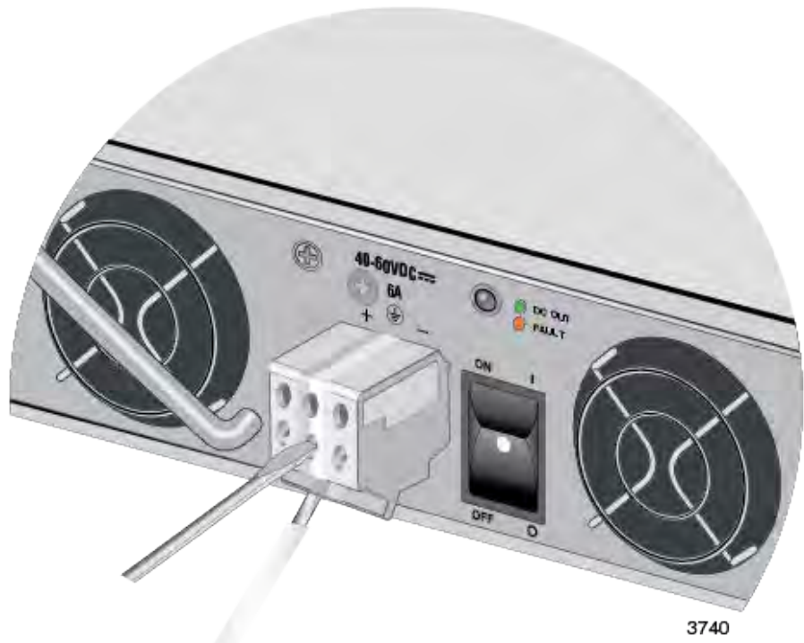
Figure 97. Disconnecting the Ground Wire to the DC Terminal Block
