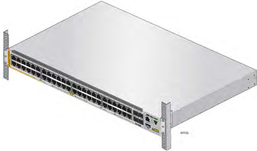
Figure 35. Switch Orientations in an Equipment Rack
