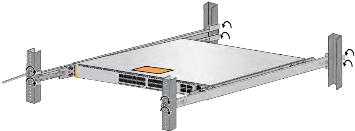
Figure 90. Tightening the Screws on the Outer Rails
