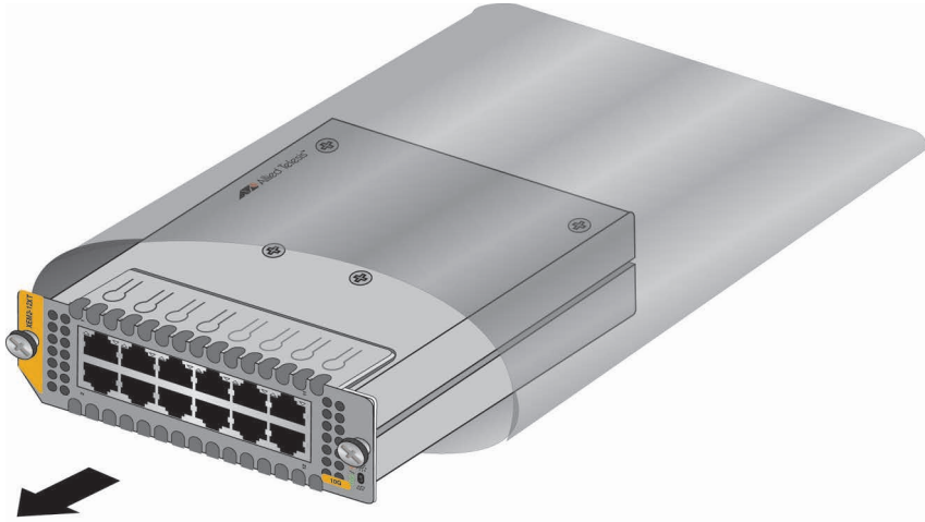
Figure 43. Removing the XEM2 Line Card from the Anti-static Bag
