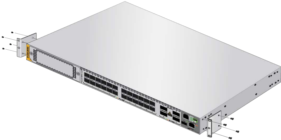
Figure 56. Attaching the Equipment Rack Brackets
