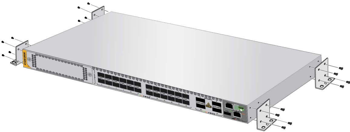
Figure 63. Installing the Brackets to the Switch for Wall Installation
