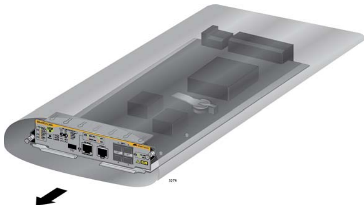
Figure 81. Removing the AT-SBx81CFC960 Controller Fabric Card from the Anti-static Bag
