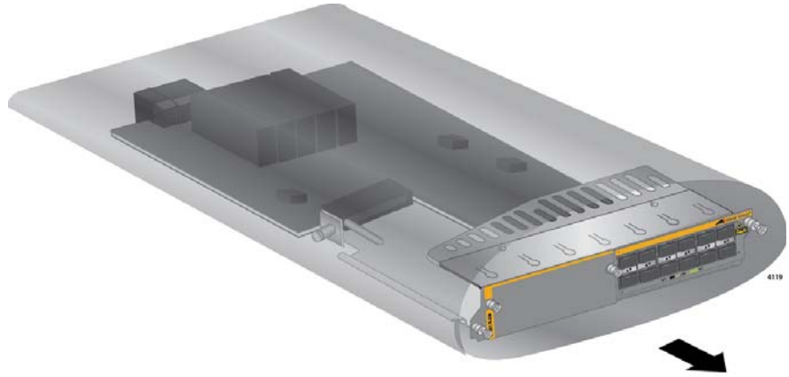
Figure 87. Removing the AT-SBx81XLEM Line Card from the Anti-static Bag
