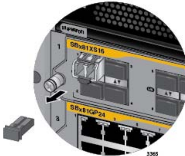
Figure 110. Removing the Dust Cover from a Transceiver
