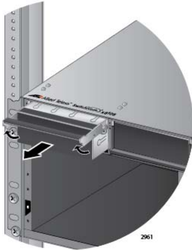
Figure 66. Removing the Blank Slot Cover from Power Supply Slot A
