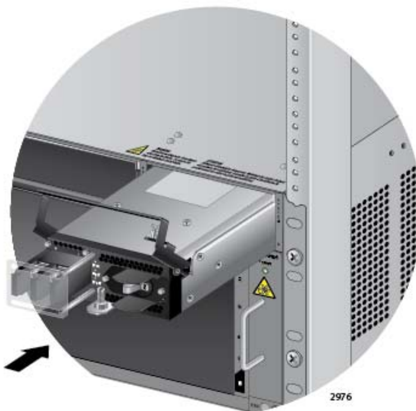
Figure 76. Inserting the AT-SBxPWRSYS1 DC System Power Supply
