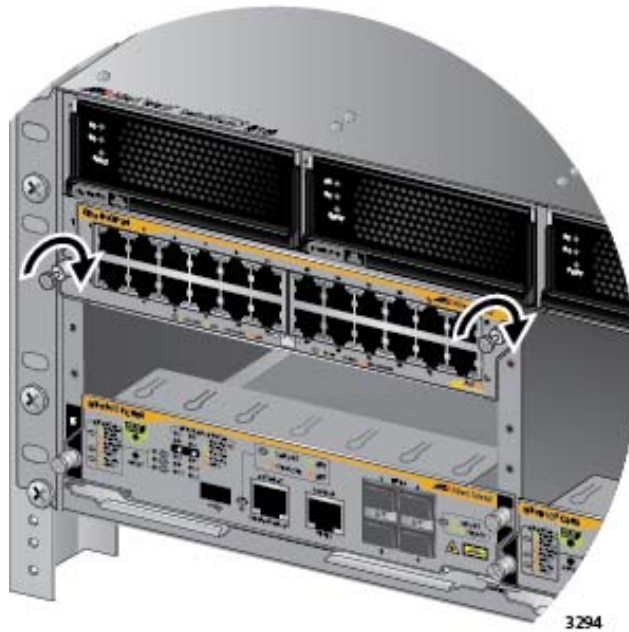
Figure 102. Tightening the Thumb Screws on an Ethernet Line Card
