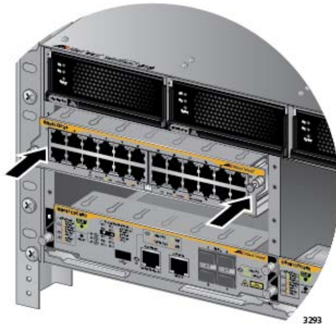
Figure 101. Seating an Ethernet Line Card on the Backplane Connector
