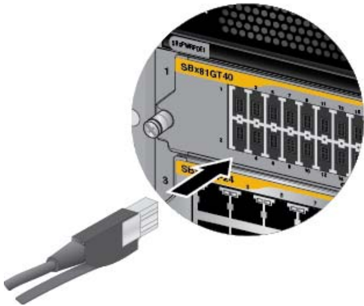
Figure 106. Connecting Cables to Ports on the AT-SBx81GT40 Line Card
