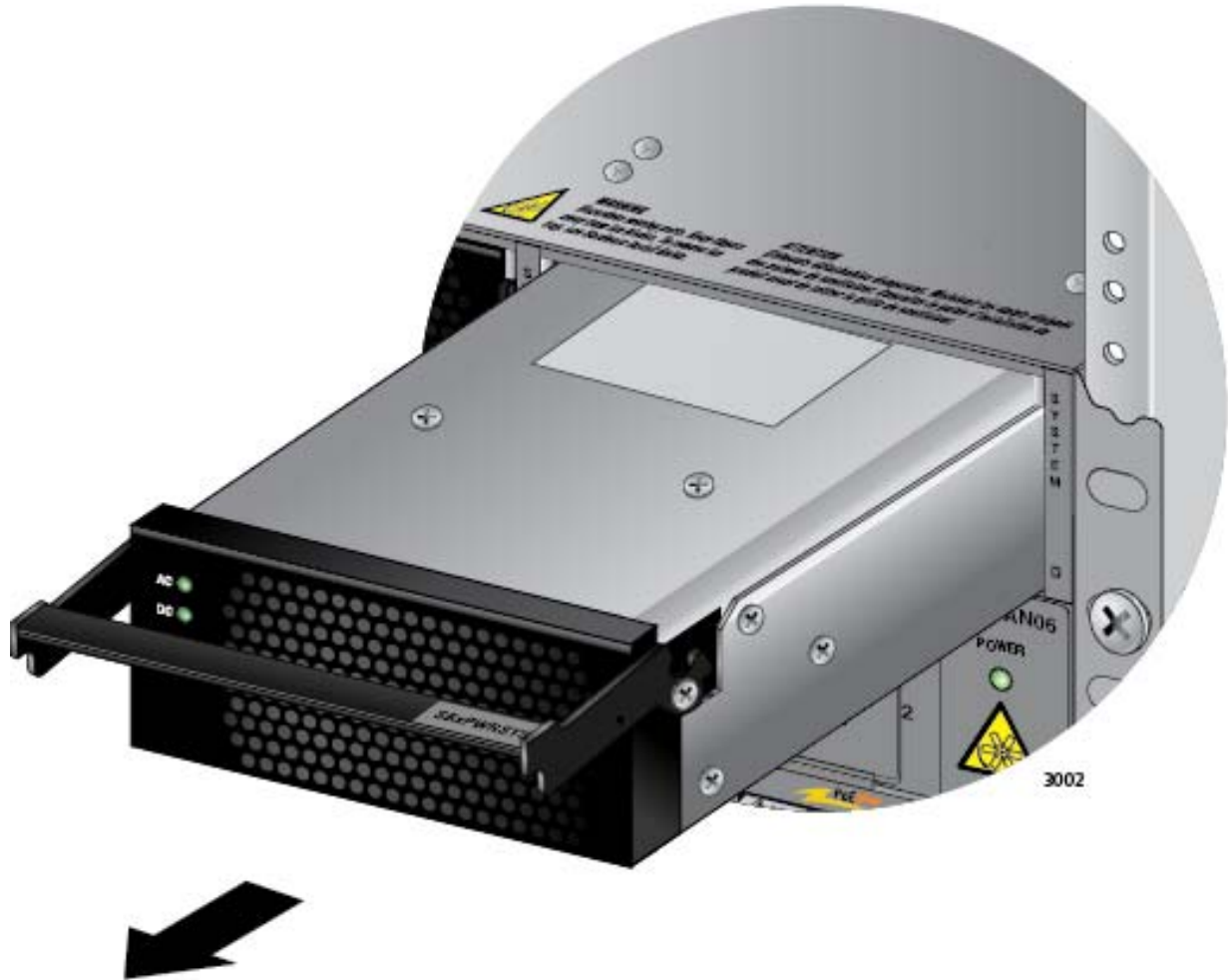
Figure 167. Removing the Power Supply from the Chassis
