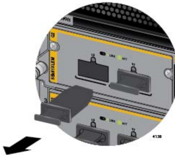
Figure 116. Removing the Dust Cover from a Slot on the AT-SBx81XLEM/Q2 Expansion Module
