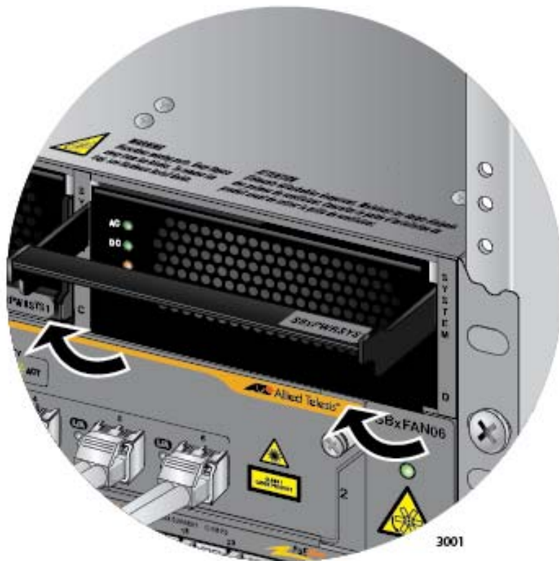
Figure 166. Lifting the Locking Handle on the Power Supply
