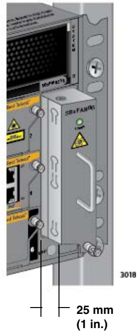
Figure 194. Withdrawing the AT-SBx81CFC960 Fan Module 25 mm (1 in.) from the Chassis
