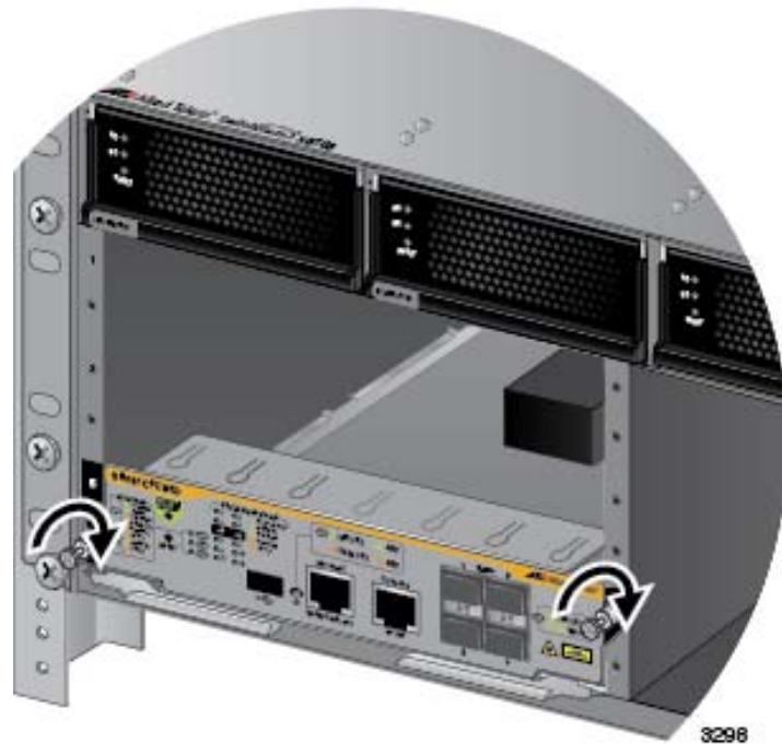
Figure 86. Tightening the Thumb Screws on the AT-SBx81CFC960 Card
