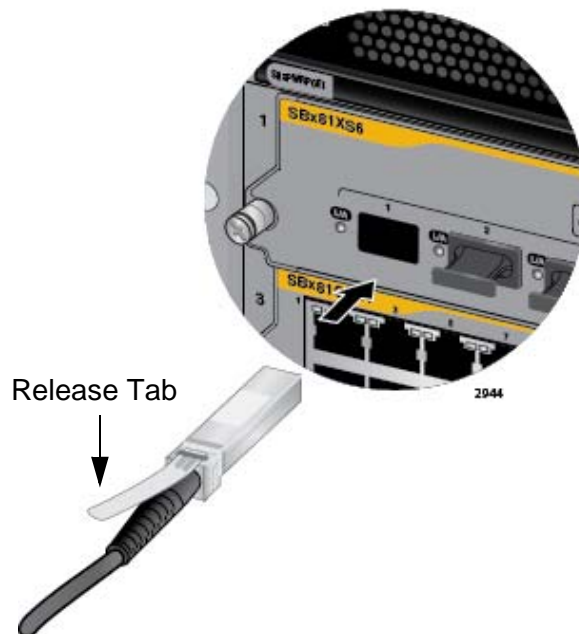
Figure 115. Installing the AT-SP10TW Cable in the AT-SBx81XS6 Line Card
