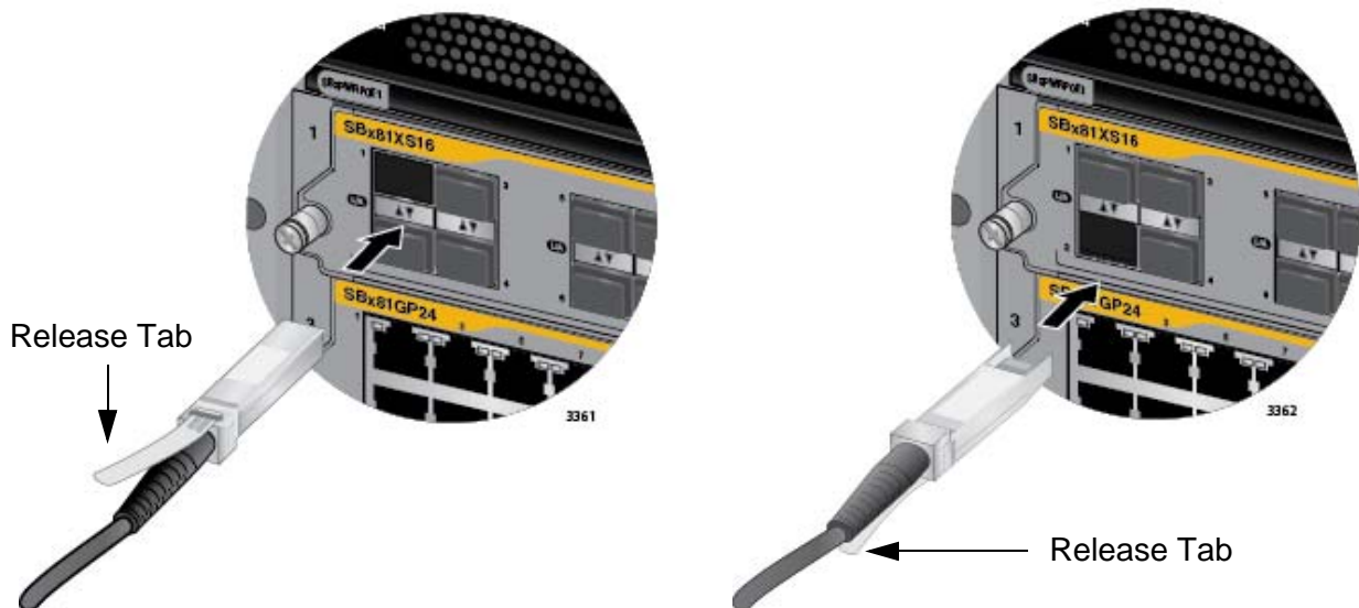
Figure 114. Installing the AT-SP10TW Cable in the AT-SBx81XS16 Line Card or AT-SBx81XLEM/XS8 Expansion Module
