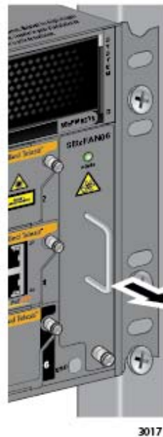
Figure 193. Loosening the AT-SBxFAN06 Fan Module from the Backplane Connector
