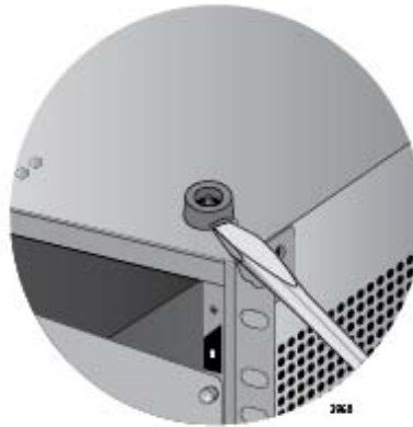
Figure 48. Removing the Rubber Feet
