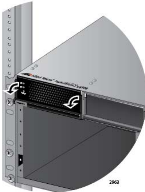
Figure 70. Locking the Handle on the AT-SBxPWRPOE1 Power Supply
