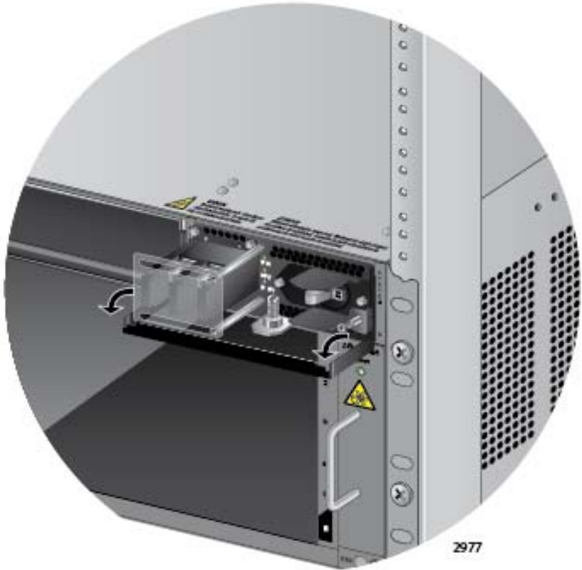
Figure 77. Locking the Handle on the AT-SBxPWRSYS1 DC System Power Supply
