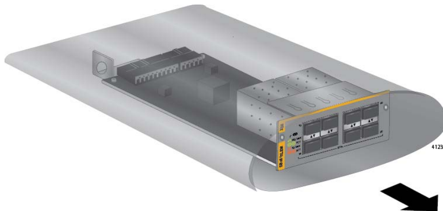
Figure 91. Removing the Expansion Module from the Anti-static Bag
