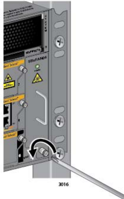
Figure 192. Loosening the Screw on the AT-SBxFAN06 Fan Module
