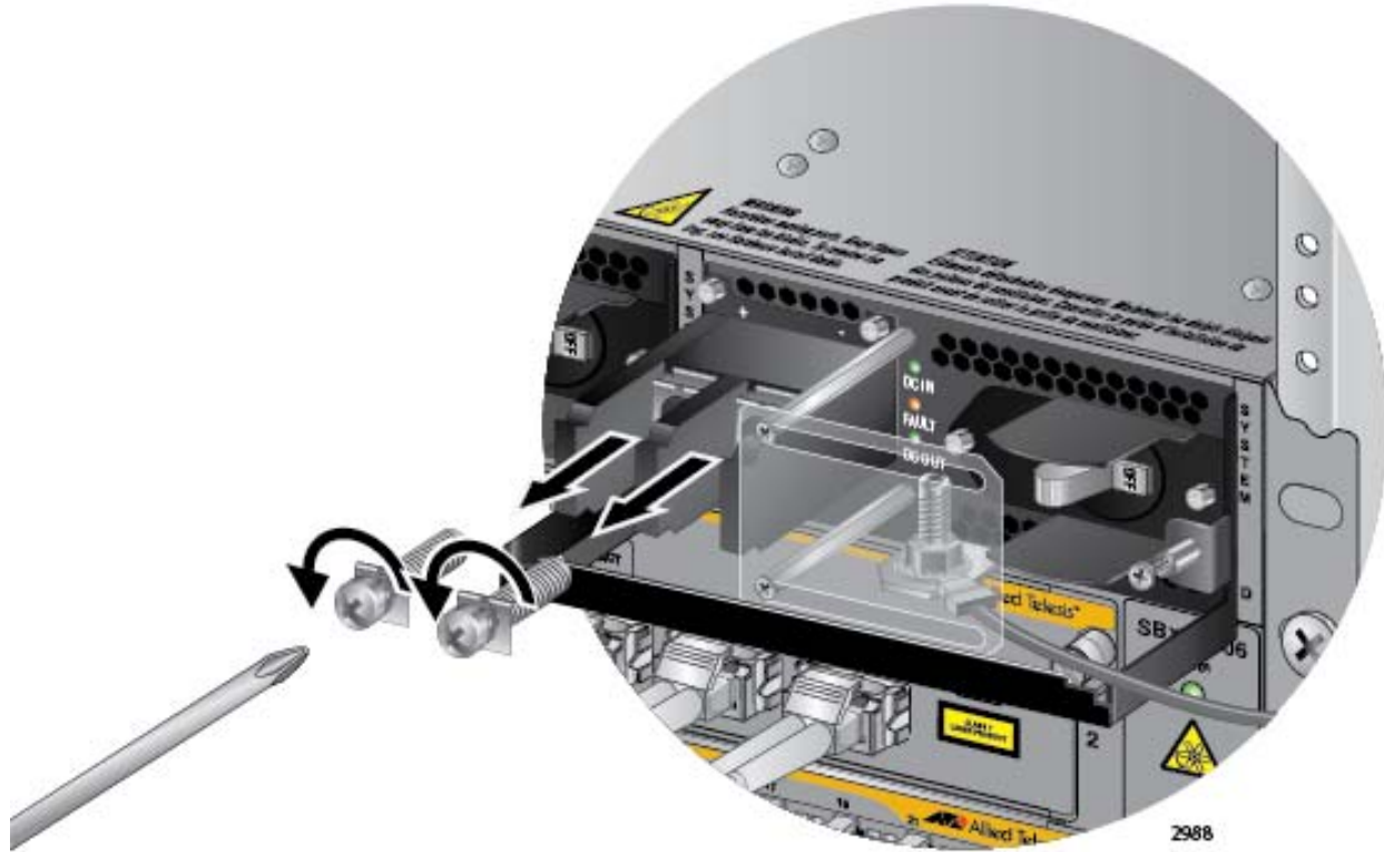
Figure 145. Removing the Terminal Screws
