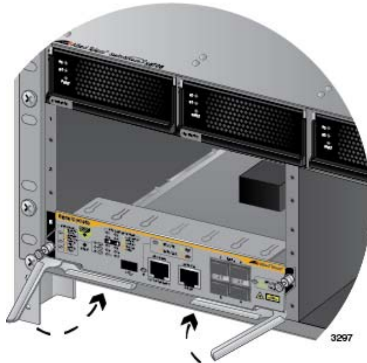
Figure 85. Closing the Locking Levers on the AT-SBx81CFC960 Controller Fabric Card
