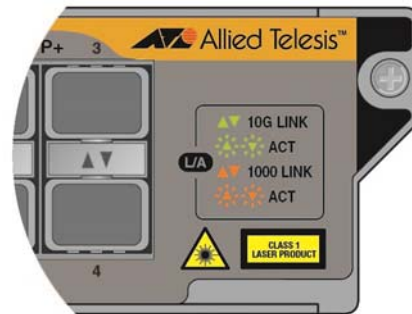
Figure 39. Legends for the SFP+ Ports on the AT-SBx81CFC960 Versions 1 and 2 Controller Cards
