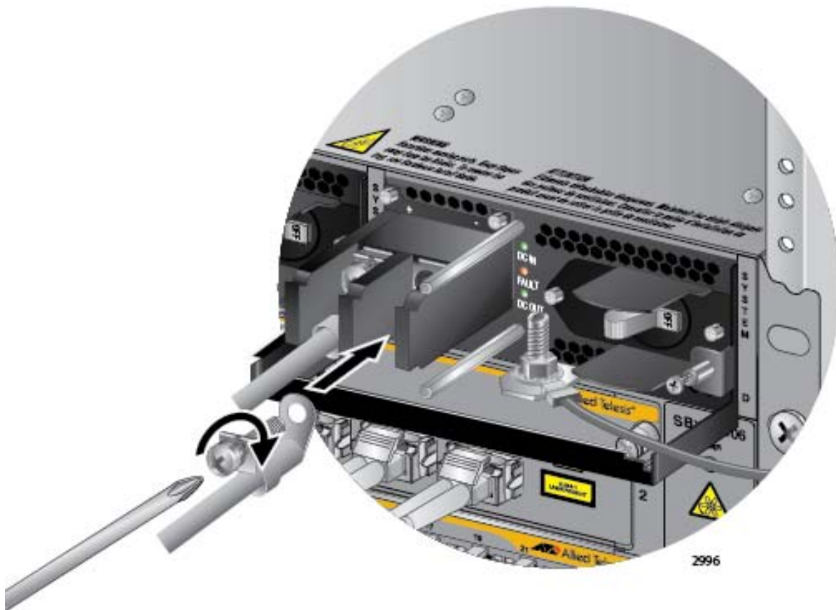
Figure 155. Connecting the Negative (-) Power Wire with a Right Angle Terminal
