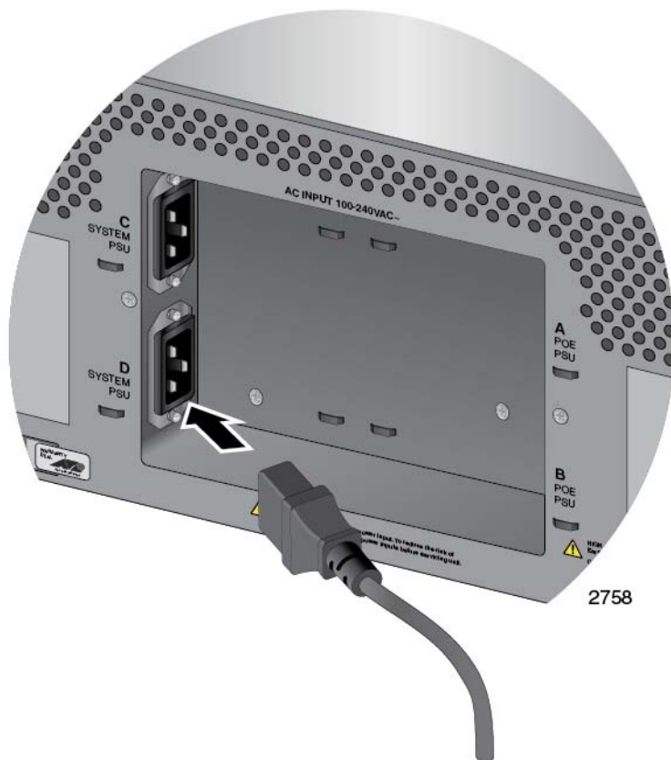
Figure 126. Connecting the AC Power Cord for the AT-SBxPWRSYS1 or AT-SBxPWRSYS2 AC System Power Supply
