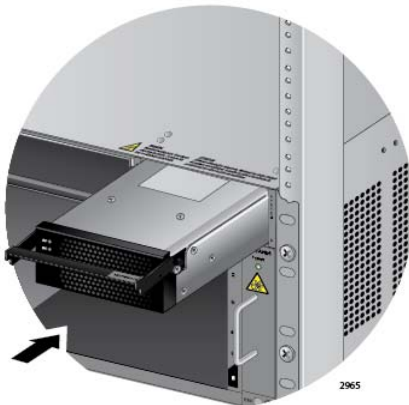
Figure 64. Inserting the AT-SBxPWRSYS1 or AT-SBxPWRSYS2 AC System Power Supply
