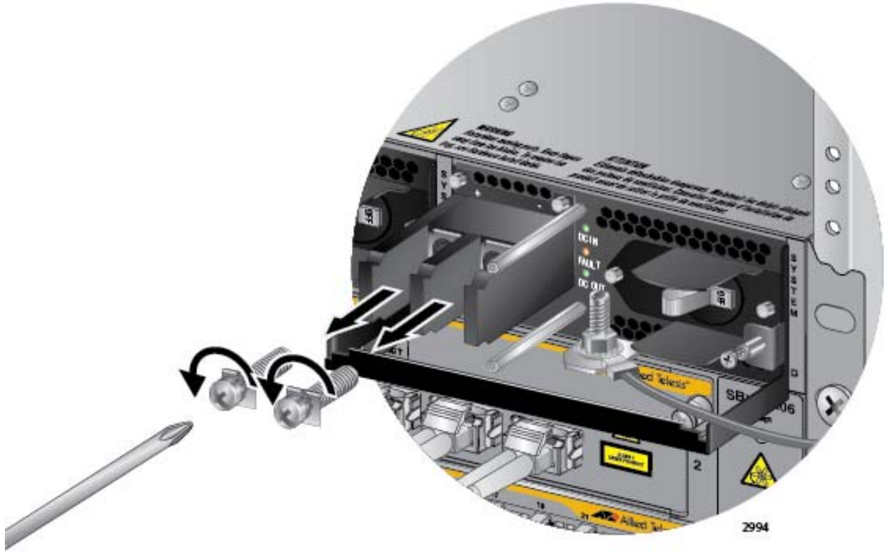
Figure 153. Removing the Terminal Screws
