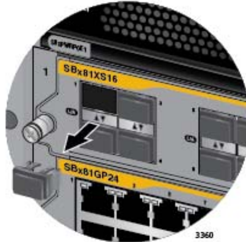
Figure 107. Removing the Dust Cover from a Transceiver Slot
