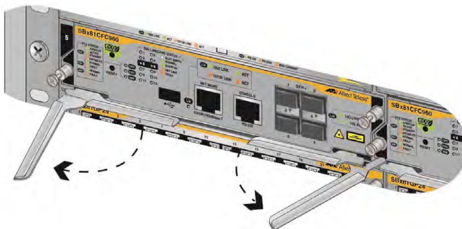
Figure 183. Pulling out the Retaining Handles on the AT-SBx81CFC960 Controller Card
