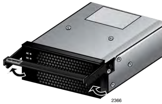
Figure 60. Unlocking the Handle on the AT-SBxPWRPOE1 Power Supply
