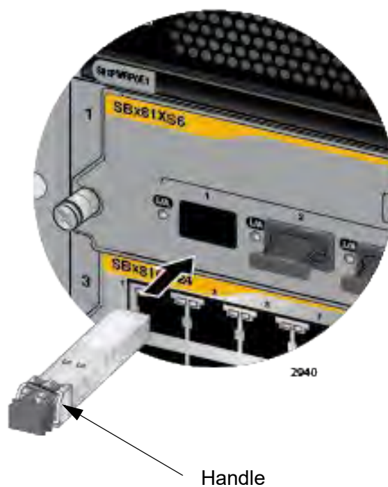
Figure 102. Installing an SFP+ Transceiver in the AT-SBx81XS6 Line Card
