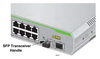
Figure 14. Positioning the SFP Handle in the Upright Position
