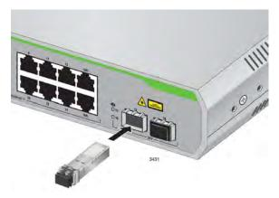
Figure 13. Inserting the SFP
